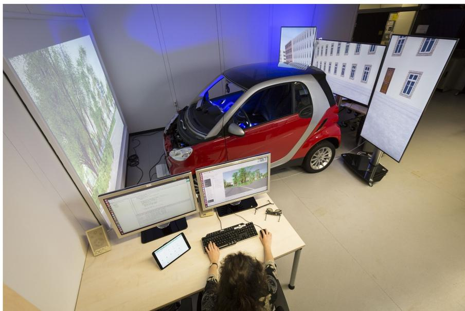
Fig. 5.6: *DriveSim* hardware setup with front projection and rear-view displays [Kal18]
