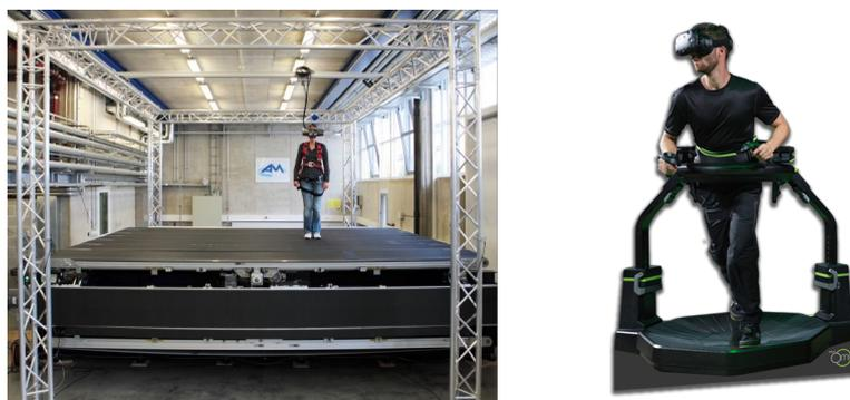
Fig. 3.5: Omnidirectional treadmills *CyberWalk* [RGSM<sup>+</sup>08] and *Virtuix Omni* [Vir20]
