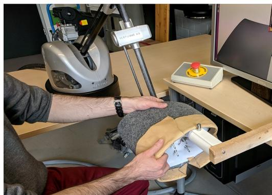
(b) Attachment of the physical mock-up of the handbag to the haptic device [Hei18]
