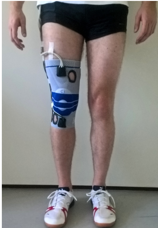
Figure 4.1: Placement of Inertial Measurement Units (IMUs) used in the study. The IMUs were positioned in the two black patch pockets at the upper and lower frontal end of the sleeve.
