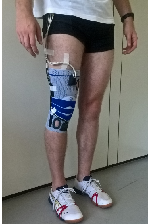
Figure 5.1: A participant wearing the knee sleeve on the right leg. The two inertial measurement units were placed in the patch pockets at the upper and lower frontal end of the knee sleeve.
