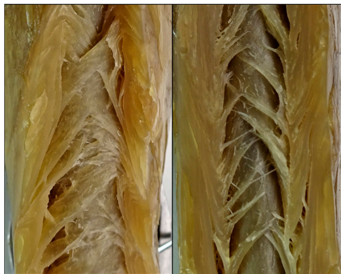
Figure 3. Product structure of extruded soy protein isolate (SPI) with material temperatures of 124 °C ( left ) and 135 °C ( right ) before cooling die. Water content (50%), screw speed (250 rpm) and mass flow (10 kg/h) were held constant. Increase in material temperature was induced by increasing the barrel temperature.
