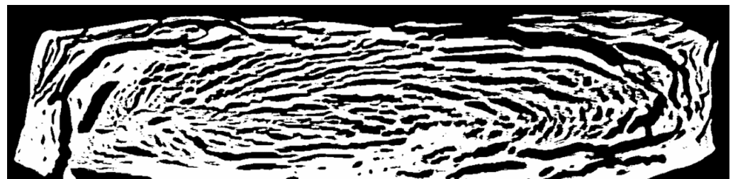
Figure 8. Microstructure of freeze-dried SPI extrudate, obtained with X-ray measurements. Sample was extruded at 50% ( w/w ) moisture content and material temperature of 124 °C before entering the cooling die. Front view is displayed. Flow direction is directed out of the image plane towards the reader.
