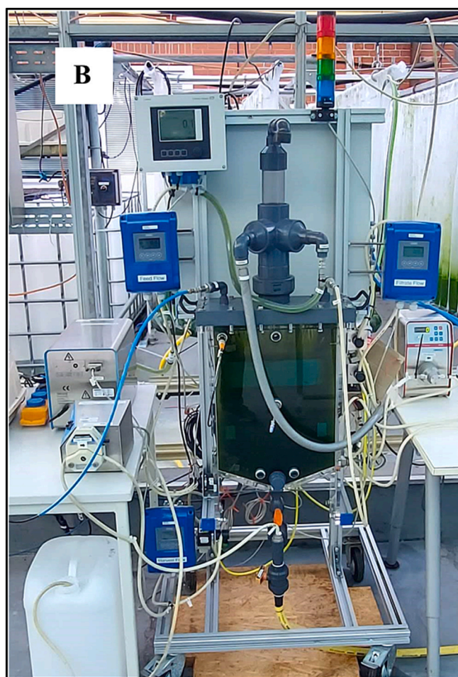
Fig. 1. A. Desmodesmus sp. cultivation and waste-water (WW) treatment in interconnected photobioreactor (PBR) system. Each PBR “bag” has a total capacity of 200L and is continuously circulated with a peristaltic pump through the entire 1000L volume of the system. Air is pumped through a porous tube running along the inside bottom of each bag that provides bubbling for mixing and gas exchange. Light is provided from natural sunlight with extra artificial light near shaded areas. Samples collected from the middle of each bag daily using a tube connected to a syringe. B: The Harvester comprising of mainly the separating chamber with hollow fiber bundles in the middle separates the algae from the WW and multiple peristaltic pumps connected to the harvester ensure their independent separation and flow rate control which allows them to be independently removed or returned to the PBR depending on the readings measured by the sensors.
