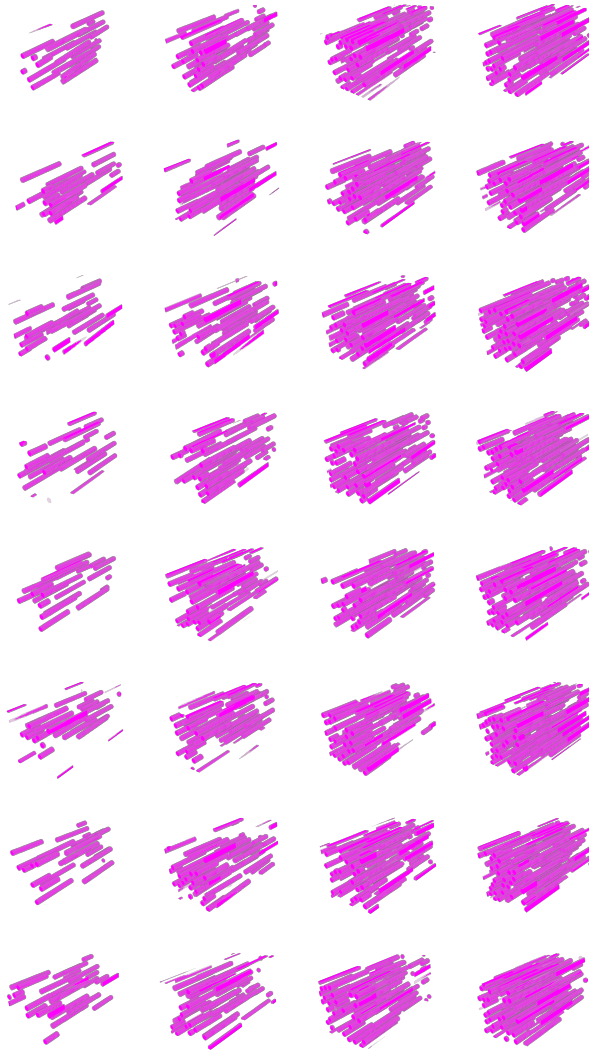
Figure A.1.1: Eight series of the investigated unidirectional synthetic microstructures. The fiber volume fractions from left to right are: 5%, 10%, 15% and 20%.
