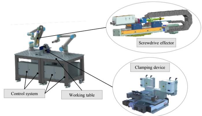
Fig. 5. Disassembly system for electric motors
