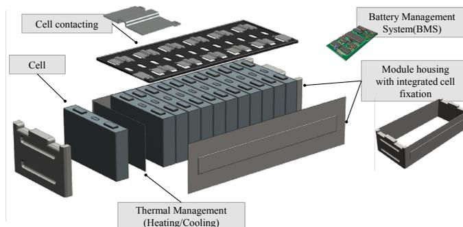
Fig. 1. Example setup of a battery module with prismatic cells
