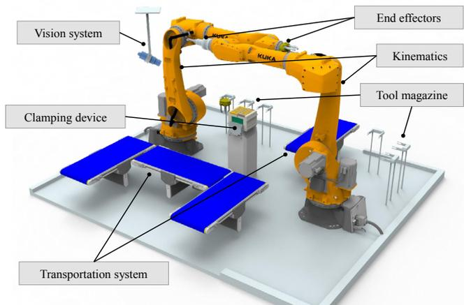
Fig. 4. Concept for a disassembly system for Li-ion modules consisting of two operation-specialized robots
