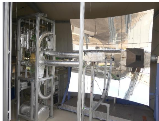
Figure 5: SOMMER test facility; left: parabolic mirror; right: liquid metal loop with thermal receiver in the focal point (Foto: F. Fellmoser)
