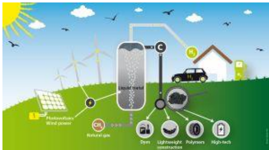
Figure 6: Methane pyrolysis by means of a bubble column reactor allows for the climate-friendly use of fossil natural gas.
