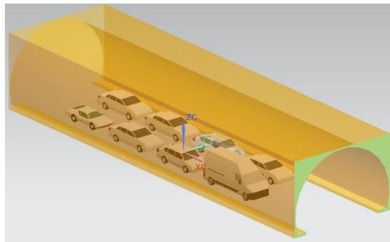
Figure 5: Tunnel segment modeled for late ignition / explosion scenario
