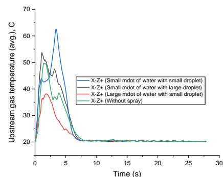
Figure 4: Gas temperature changes in upstream caused by water spray
