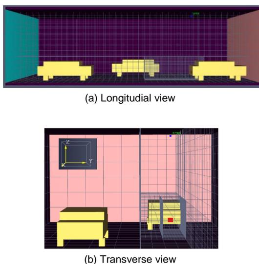
Figure 3: Numerical mesh of the simulated road tunnel segment with 3 cars, one of them (on the right hand side) releasing hydrogen through a nozzle (red dot)
