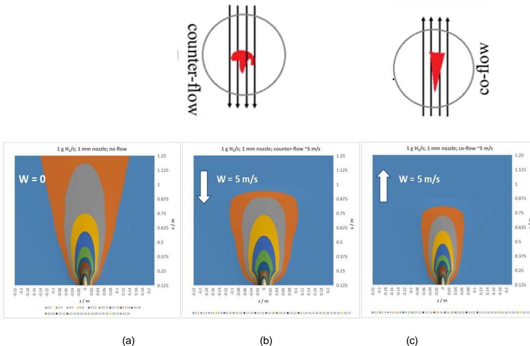
Figure 2: Measured concentrations in horizontal plane at height of release nozzle; (a) without ventilation, (b) with counterflow ventilation (c) with co-flow ventilation
