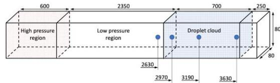
Figure 8: Experimental set-up for the Chauvin experiments
