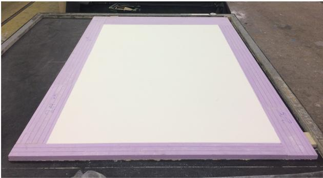
(a) Internal construction of a VIP cooling box wall.
