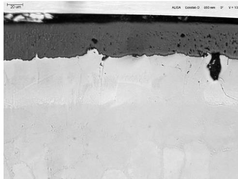
850 mm: ZrO<sub>2</sub> 44 µm; α-Zr(O) 60 µm
