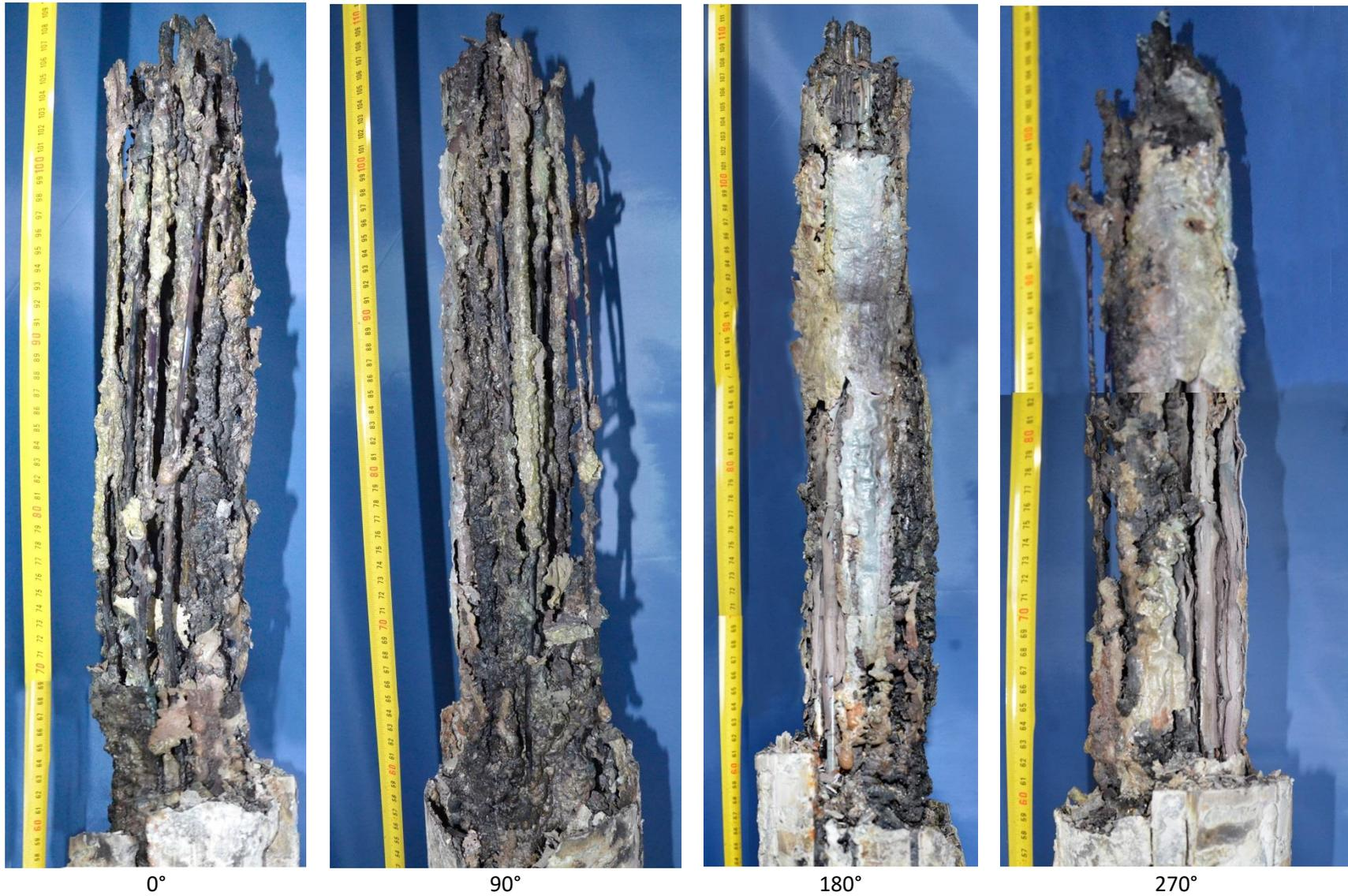
**Figure 71** QUENCH-18; Post-test bundle overview between about 550 and 1100 mm at four angle positions.
