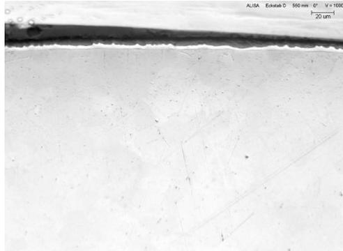
550 mm: ZrO<sub>2</sub> 5 µm; α-Zr(O) 3 µm
