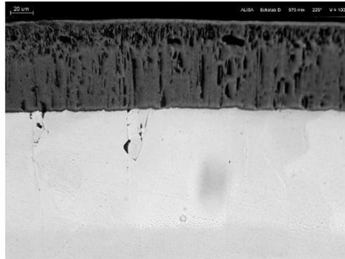
975 mm: ZrO<sub>2</sub> 79 µm; α-Zr(O) 105 µm
