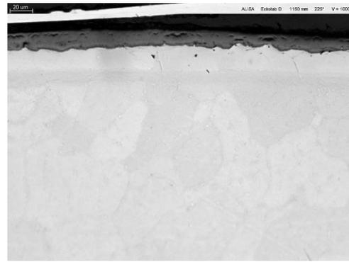
1150 mm: ZrO<sub>2</sub> 15 µm; α-Zr(O) 23 µm
