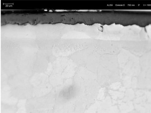
750 mm: ZrO<sub>2</sub> 27 µm; α-Zr(O) 31 µm
