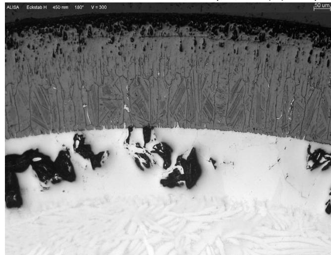
450 mm: no nitrides, ZrO<sub>2</sub> 340 μm, α-Zr(O) 208 μm
