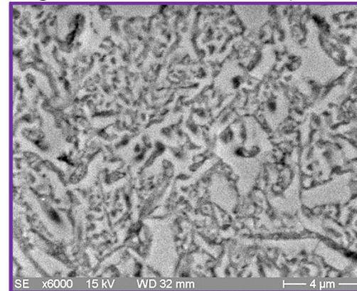
SEM image and EDX spectrum of zirconium oxides and nitrides porous area
