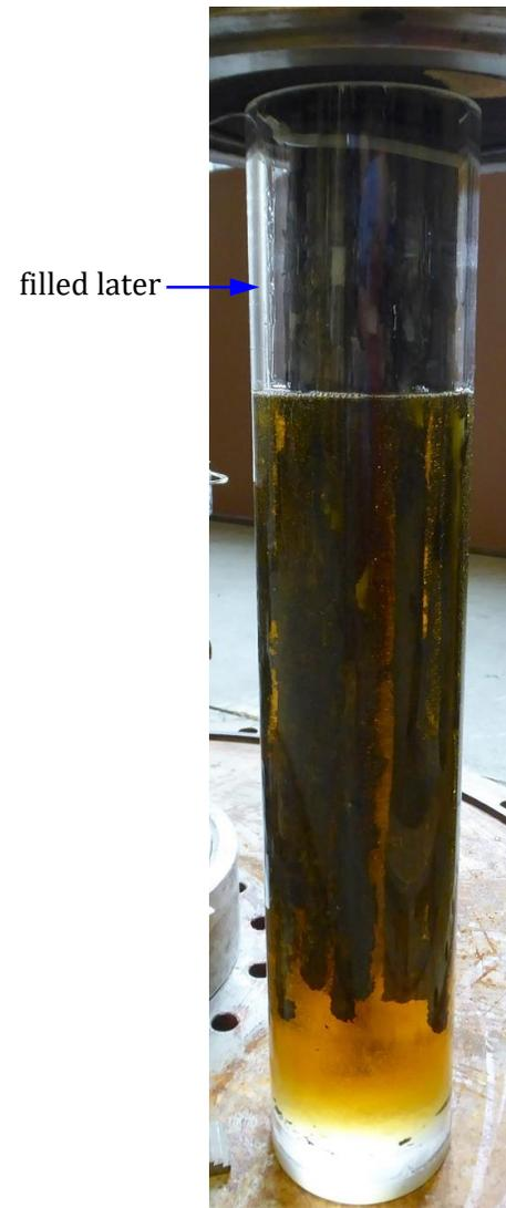
upper bundle part (without rods 3 and 23) embedded in epoxy
