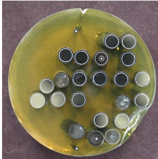
1480 mm: intact rods, slightly oxidized clads
