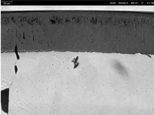
950 mm: ZrO<sub>2</sub> 81 µm; α-Zr(O) 108 µm
