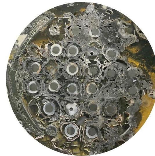
560 mm: melt collection inside grid spacer
