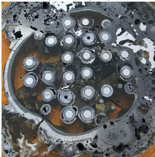
350 mm: local molten pool at bundle periphery formed by relocated molten shroud
