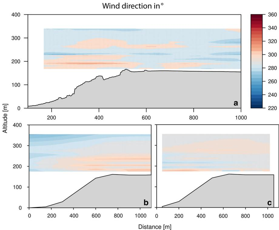
**Fig. 8** MASC-3 measurement of the wind direction derived through interpolation from horizontal flight legs between 1255–1417 UTC (a) and the mean wind speed during the UAS flight time calculated by WRF (b) and OpenFOAM (c) models on the 22 September 2018. The left side of the plot is facing west. Reference height of zero is at the bottom of the valley
