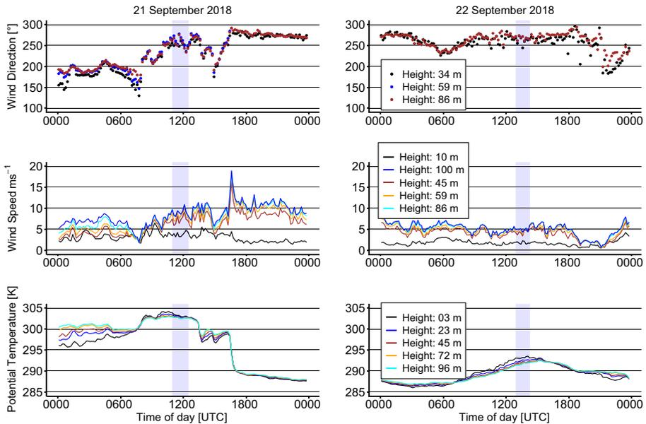
**Fig. 4** Mean wind speed and wind direction (10, 34, 45, 59, 86, and 100 m) measured by cup anemometer and wind vanes and a Thies thermometer (3, 23, 45, 72, and 96 m) mounted on the wind measurement mast close to the escarpment on 21 September and 22 September 2018. The blue vertically stretched rectangles indicate the flight duration of the UAS
