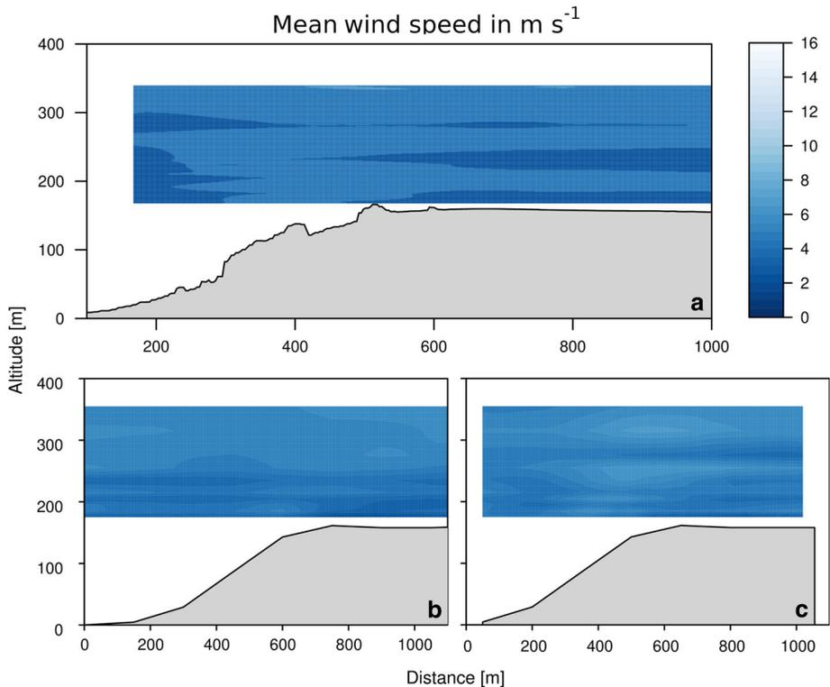
**Fig. 6** MASC-3 measurement of the mean wind speed derived through interpolation from horizontal flight legs between 1255–1417 UTC (a) and the mean horizontal wind speed during the UAS flight time calculated by WRF (b) and OpenFOAM (c) models on 22 September 2018. The left side of the plot is facing west. Reference height of zero is at the bottom of the valley
