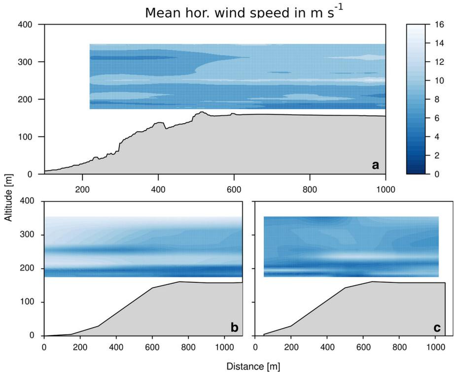
**Fig. 5** MASC-3 measurement of the mean wind speed derived through interpolation from horizontal flight legs between 1055–1229 UTC (a) and the mean horizontal wind speed during the UAS flight time calculated by WRF (b) and OpenFOAM (c) models on 21 September 2018. The left side of the plot is facing west. Reference height of zero is at the bottom of the valley
