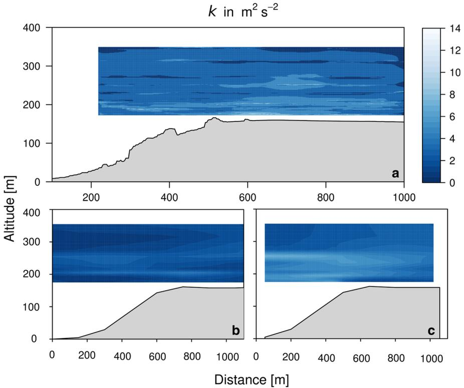
**Fig. 9** MASC-3 measurement of the TKE derived through interpolation from horizontal flight legs between 1055–1229 UTC (a) and the mean wind speed during the UAS flight time calculated by WRF (b) and OpenFOAM (c) models on 21 September 2018. The left side of the plot is facing west. Reference height of zero is at the bottom of the valley
