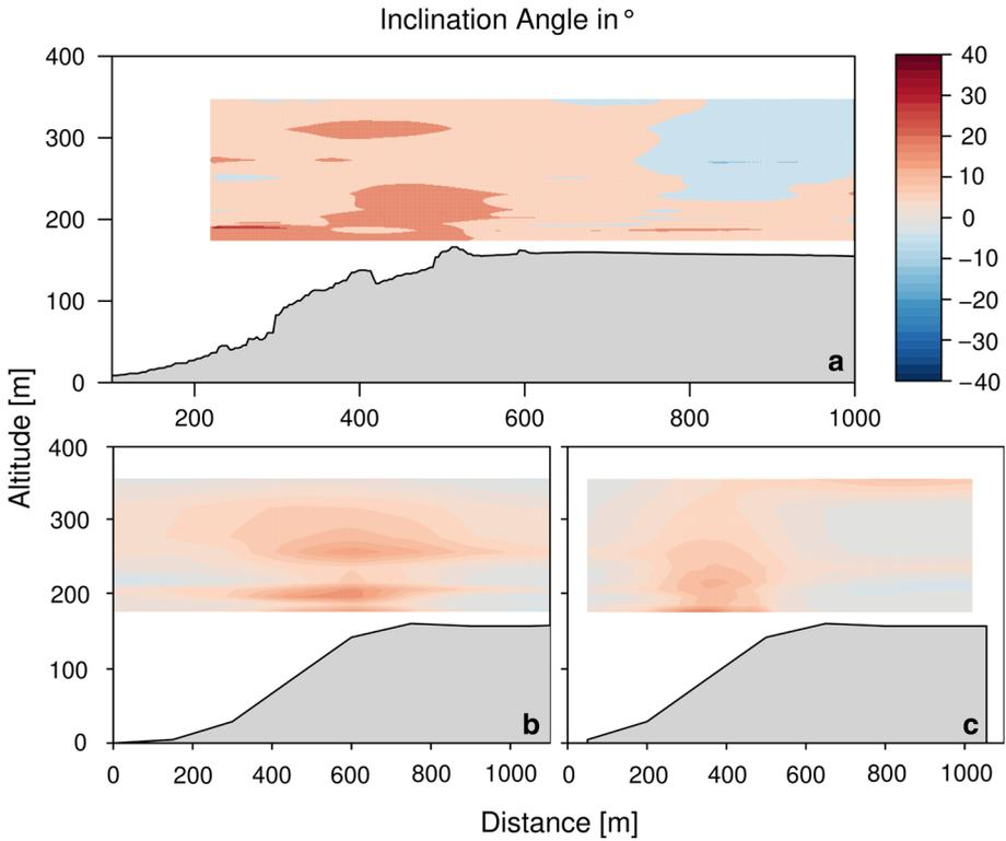
**Fig. 11** MASC-3 measurement of the inclination angle derived through interpolation from horizontal flight legs between 1055–1229 UTC (a) and the mean wind speed during the UAS flight time calculated by WRF (b) and OpenFOAM (c) models on 21 September 2018. The left side of the plot is facing west. Reference height of zero is at the bottom of the valley
