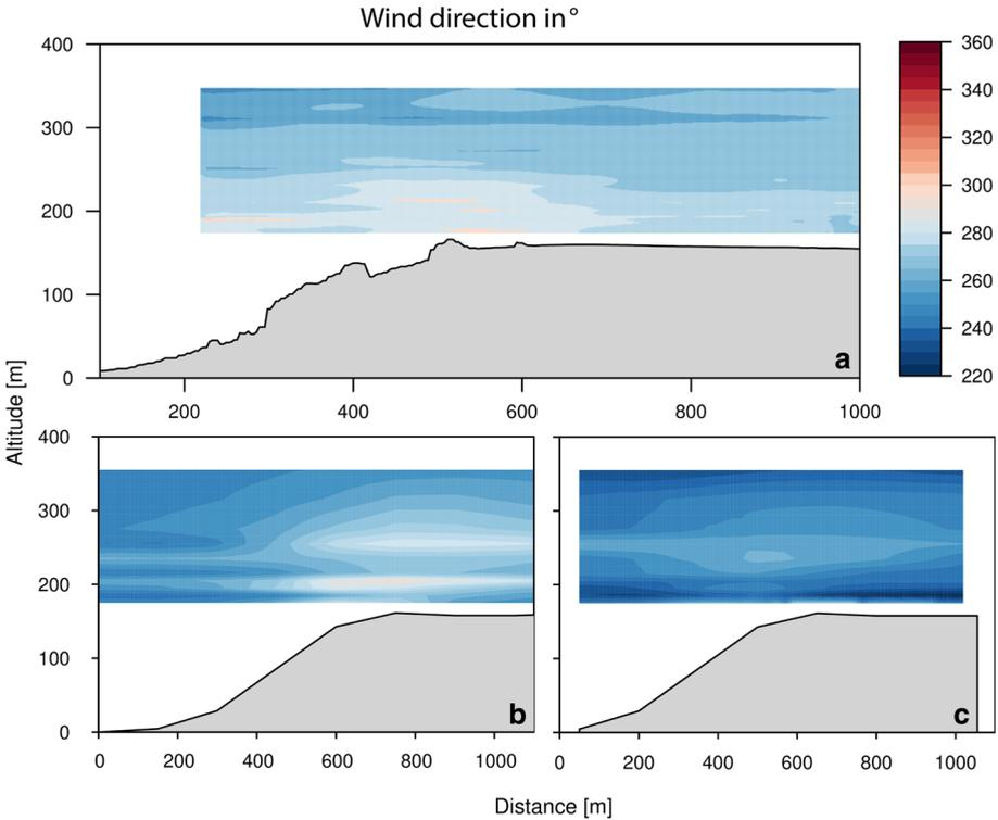
**Fig. 7** MASC-3 measurement of the wind direction derived through interpolation from horizontal flight legs between 1055–1229 UTC **(a)** and the mean wind speed during the UAS flight time calculated by WRF **(b)** and OpenFOAM **(c)** models on 21 September 2018. The left side of the plot is facing west. Reference height of zero is at the bottom of the valley
