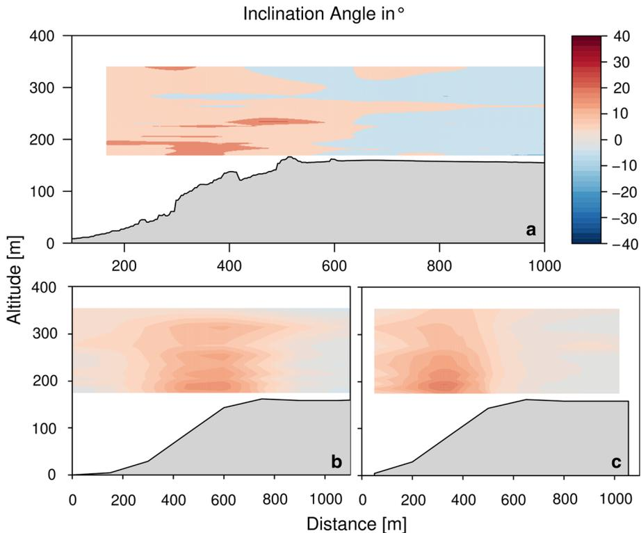
**Fig. 12** MASC-3 measurement of the inclination angle derived through interpolation from horizontal flight legs between 1255–1417 UTC (a) and the mean wind speed during the UAS flight time calculated by WRF (b) and OpenFOAM (c) models on 22 September 2018. The left side of the plot is facing west. Reference height of zero is at the bottom of the valley
