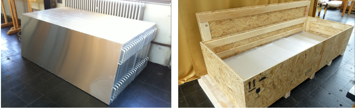
Figure 5.17: Left: Shown is the space saving transport possibility via a stacking of the IceScint detectors. The bottom side of one detector is protected from scratching during shipment by small wooden beams with the top side of the next detector. Right: One of the constructed transport crates for shipping. There is room for 8 detectors in each transport crate.
