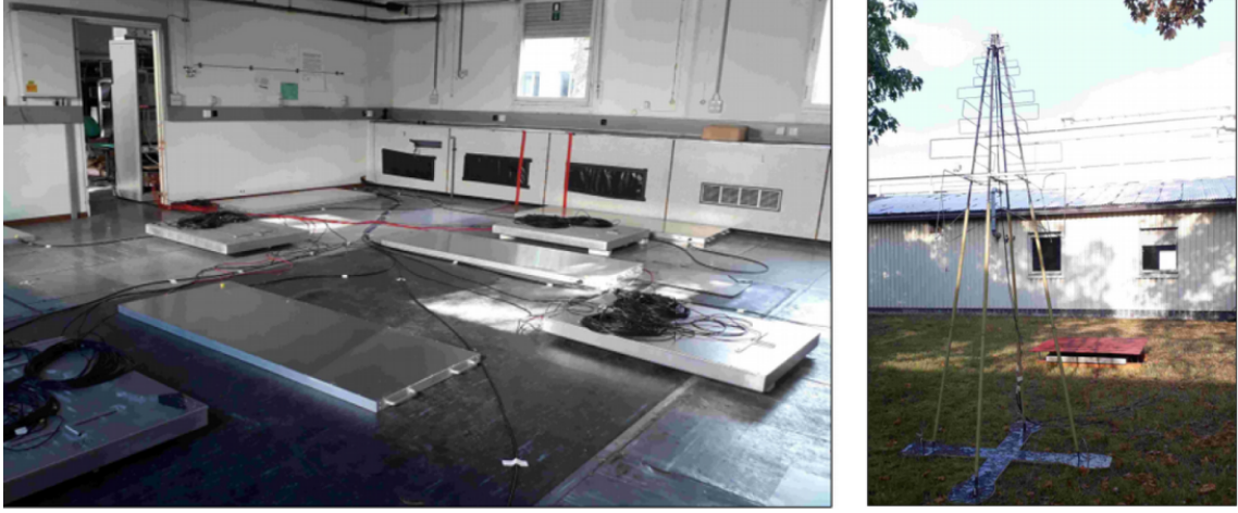
Figure 8.2: Left: Inside the barrack. Visible are eight IceScint detectors and four Mini-KASCADE detector housings with 2 detectors each. The DAQ, IceTAXI for IceScint and KAFE for Mini-KASCADE, is in another room of the barrack, visible behind the open door top left left of the picture. Right: Photo of one of the SKA antennas in front of the barrack with the mechanical structure as used in season 2018/19.
