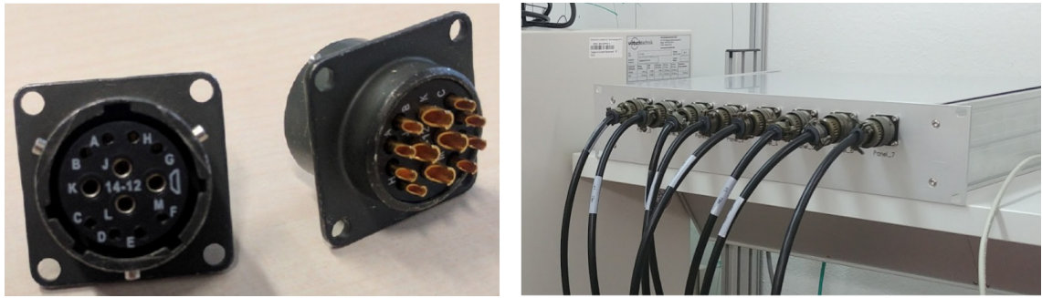
Figure 5.11: Left: Picture of the used Amphenol Co. Ltd. PT-Series connectors. This military standard is widely used for several experiments in Antarctica and was recommended by IceCube. Right: The IceTAXI frame with 8 connected IceScint detectors in the SPOCK lab for hodoscope measurements. It shows the male and female part of the Amphenol connectors, including the stiff Cat 7 cable from Draka Co. Ltd.
