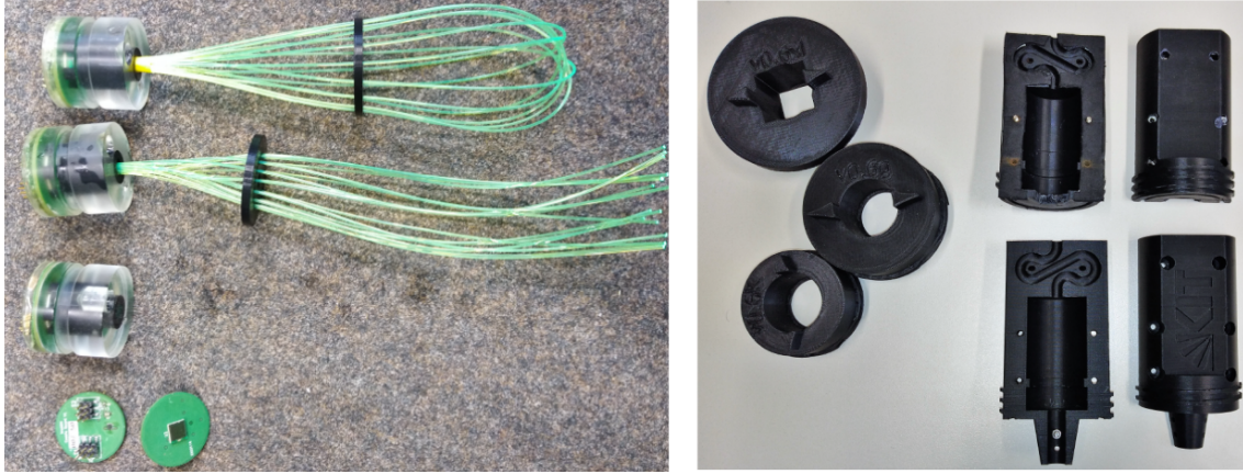
Figure 10.7: Left: Picture of the different readouts of the SiPM and the different optical fiber setups to investigate the light yield produced by Cherenkov light. Right: Developed holder for the glued cookie with the SiPM and the optical fiber. In addition it serves as photon shielding and easy system to attach and detach different optical fiber setups by an integrated thread which fits to the thread of the used coffee cans.
