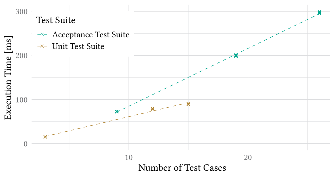
Figure 5.4: Execution time measurements for the acceptance test suite (green) and the unit test suite (brown). The linear regressions are superimposed with dashed lines.
