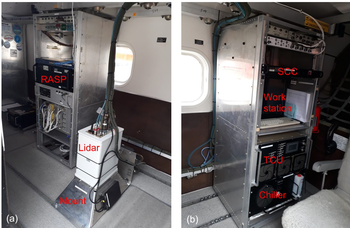
Fig. 6.1.: Prototype ADL installation inside the Dornier 128-6 aircraft used for the research flights analyzed in this work. (a) Lidar transceiver mounted on the aircraft floor, pointing along the aircraft vertical axis through an opening. Real-time advanced signal processing (RASP) unit for data acquisition mounted in rack. (b) Operator position. Mounted in rack are: work station to control all components, system control computer (SCC), transceiver control unit (TCU) and chiller for lidar cooling (Chiller).
