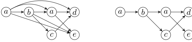
Figure 3.1: The Dependence Graph (left) and Hasse Diagram (right) for the trace [abcaed] according to the trace monoid \mathbb{M}(A, Z) over the alphabet A = \{a, b, c, d, e\} and independencies Z = \{(a, c), (c, a), (b, d), (d, b), (d, e), (e, d)\} .
