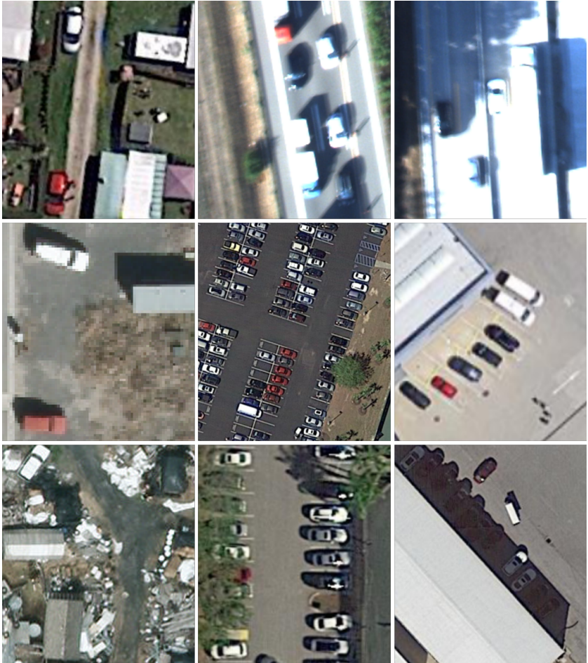
Figure 1.2: Illustration of typical challenges occurring in aerial imagery. First row: image noise 1 , motion blur 2 and illumination 2 . Second row: low resolution 3 , high intra-class variance 3 and low inter-class variance 1 . Third row: intricate background 3 , partial occlusion 1 and shadow 1 .
