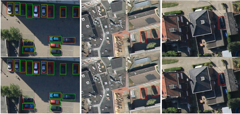
Figure 8.7: Qualitative detection results (red boxes) and corresponding GT (green boxes) for EMT-MFD Faster R-CNN with VGG16 (top row) and with ZynqNet (bottom row) on the ITCVD dataset show the good detection accuracy. Note that even multiple vehicles with missing annotations are correctly detected.
