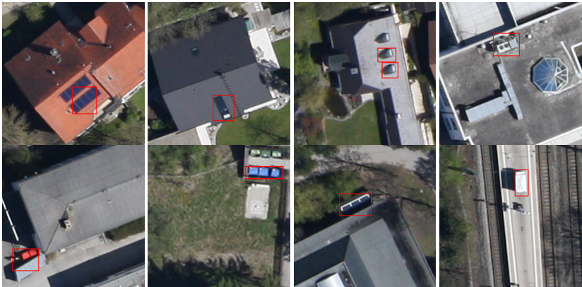
Figure 3.4: Qualitative detection results on the DLR 3K dataset that highlight the effect of the performed adaptations. False alarms due to the exploitation of shallow layers as feature map are mainly caused by objects with vehicle-like shapes such as solar cells or windows on buildings.
