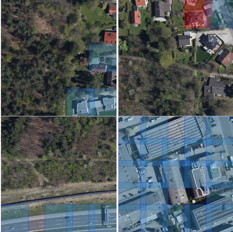
Figure 7.9: Classification results of the SAR module on DLR 3K. Highlighted regions are classified as region that contain at least one object and are considered for detection. Regions labeled in blue contain vehicles, whereas regions labeled in red contain no vehicles.
