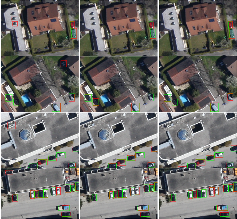
Figure 8.4: Qualitative detection results (red boxes) and corresponding GT (green boxes) for Faster R-CNN with VGG16 (left column), EMT-MFD Faster R-CNN + SAR with VGG16 (middle column) and EMT-MFD Faster R-CNN + SAR with ZynqNet (right column) on DLR 3K demonstrate that the proposed approaches are more robust to false alarms due to vehicle-like structures.
