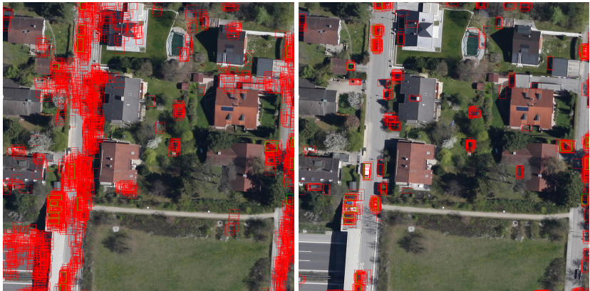
Figure 5.15: Region proposals (red boxes) for a mean anchor box area of 256^2 pixels (left) and 28^2 pixels (right) that are forwarded to the classification stage as well as the corresponding GT (green boxes). Note that only region proposals with a confidence score above 0.5 are depicted.
