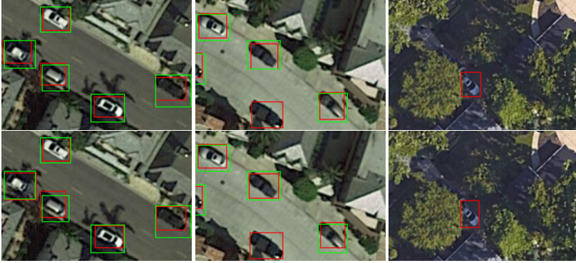
Figure 8.10: Qualitative detection results (red boxes) and corresponding GT (green boxes) for EMT-MFD Faster R-CNN with VGG16 (top row) and with ZynqNet (bottom row) on the DOTA dataset indicate the good detection accuracy in unseen images from different sensors. Note that even multiple vehicles with missing annotations are correctly detected.
