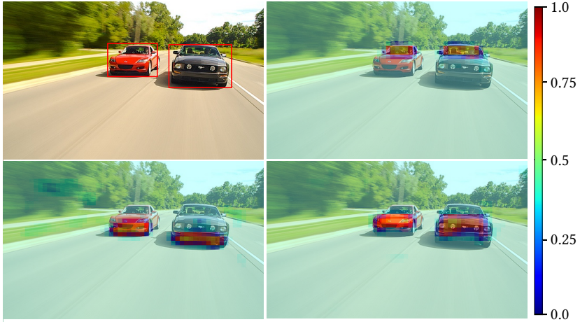
Figure 5.4: Activations of three filters from conv5_3 used as feature map and the corresponding detection results on PASCAL VOC indicate that the feature map resolution is sufficient to accurately localize objects. The activations are normalized to values between 0 and 1.
