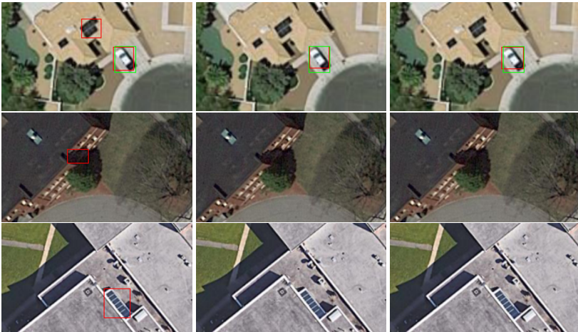
Figure 8.11: Qualitative detection results (red boxes) and corresponding GT (green boxes) for Faster R-CNN with VGG16 (left column), EMT-MFD Faster R-CNN with VGG16 (middle column) and EMT-MFD Faster R-CNN with ZynqNet (right column) on the DOTA dataset demonstrate that the proposed approaches are more robust to false alarms due to vehicle-like structures in unseen data.
