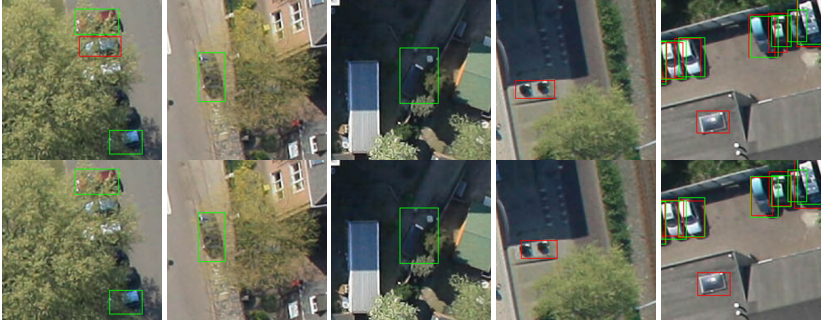
Figure 8.9: Qualitative examples of missed detections and false alarms for EMT-MFD Faster R-CNN with VGG16 (top row) and ZynqNet (bottom row) on the ITCVD dataset. Missed detections are mainly due to objects that are partially occluded, e.g., by trees, or that are located in shadowed areas, while false alarms are mostly caused by structures located on asphalted areas.
