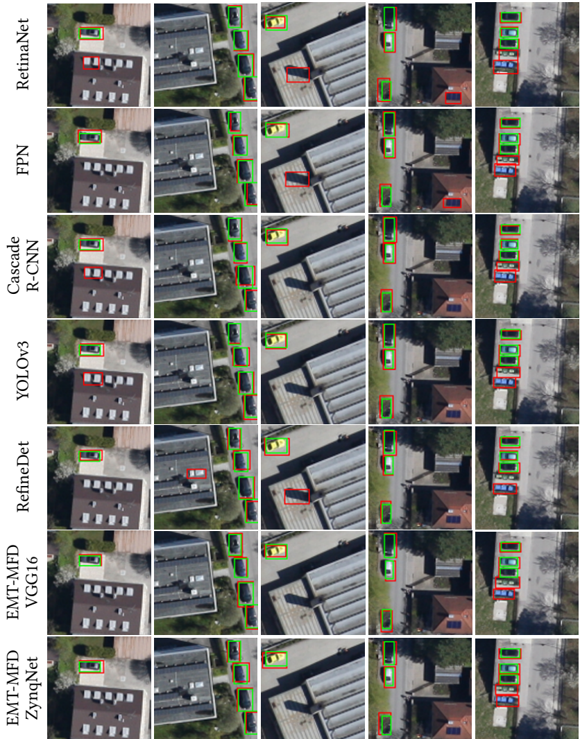
Figure 8.5: Qualitative detection results (red boxes) and corresponding GT (green boxes) for EMT-MFD Faster R-CNN + SAR with VGG16 and ZynqNet, respectively, and representative existing work on DLR 3K with a GSD of 26 cm.
