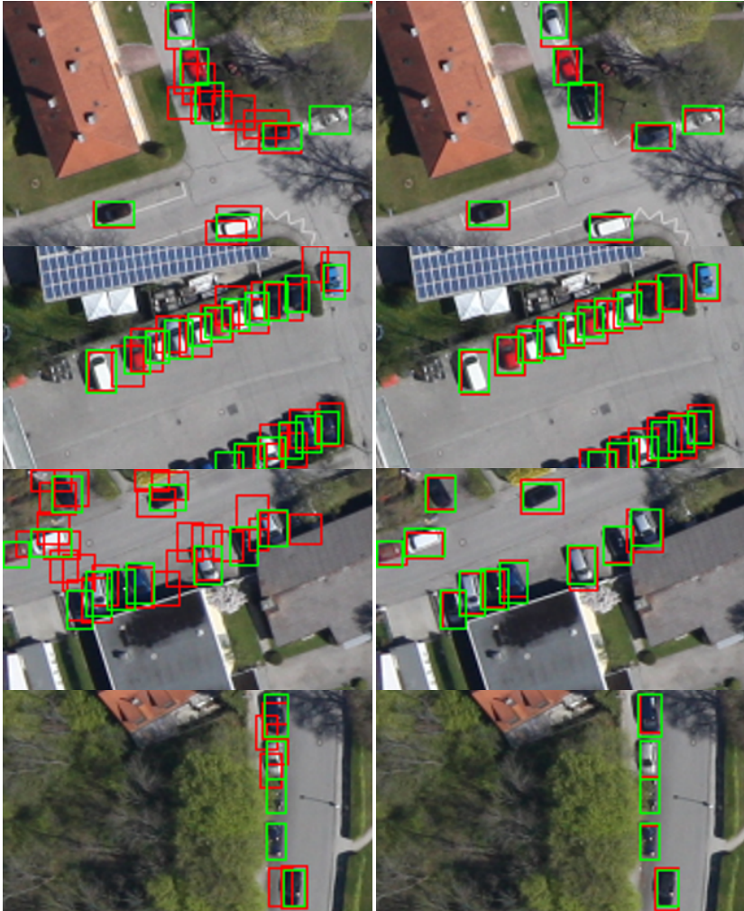
Figure 5.18: Qualitative detection results (red boxes) for Faster R-CNN using conv5_3 (left) and conv3_3 (right) as feature map and the corresponding GT (green boxes) for a GSD of 26 cm. The higher feature map resolution results in better localized detections and thus, considerably fewer false positive detections. Furthermore, the number of missed detections is clearly reduced. Remaining false negative detections in case of conv3_3 are mainly due to heavy occlusions, e.g., caused by trees (bottom row).
