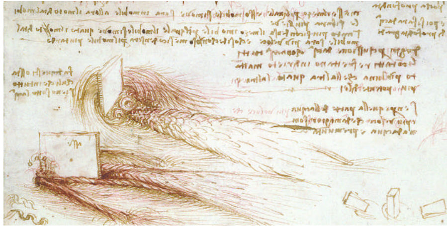
Figure 4.1: Visualization of a turbulence wake as water streams past an obstacle, drawn by Leonardo da Vinci [207].
