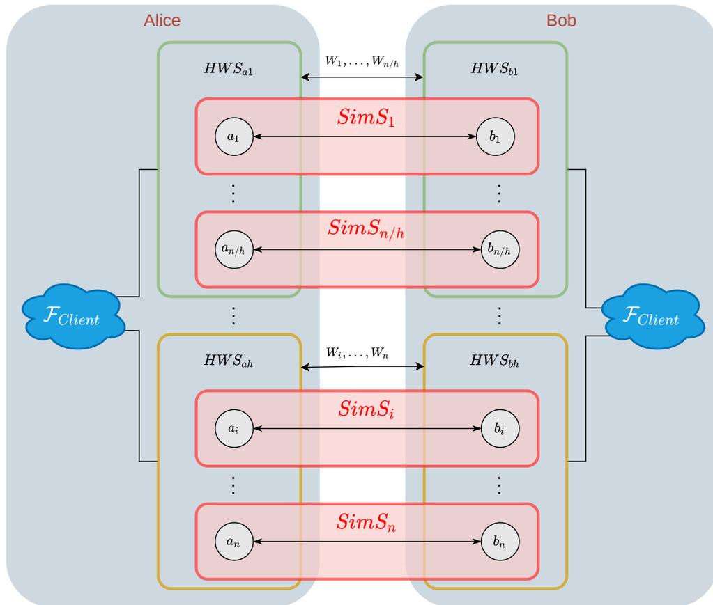
Figure 5.3: Overview of the compiled protocol, each party consists of several HWS of different colors. HWS run the inner protocol clients (the  $a$ s and  $b$ s) that simulate  $SimS$  together. HWS of different parties that simulate  $SimS$  together and check each others watchlists  $W_i$  have the same color. Note that for readability the interface client, from which the HWS receive input and output is not shown here.
