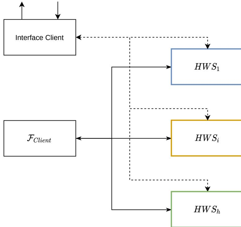
Figure 5.2: The layout of a single party in the combined protocol with an interface client for input and output, several HWS in different colors and the ideal client functionality.
