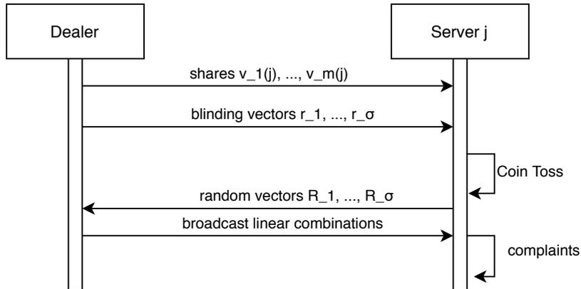
Figure 6.2: The VSS scheme used in the combined protocol. The scheme was proposed in [IPS10].
