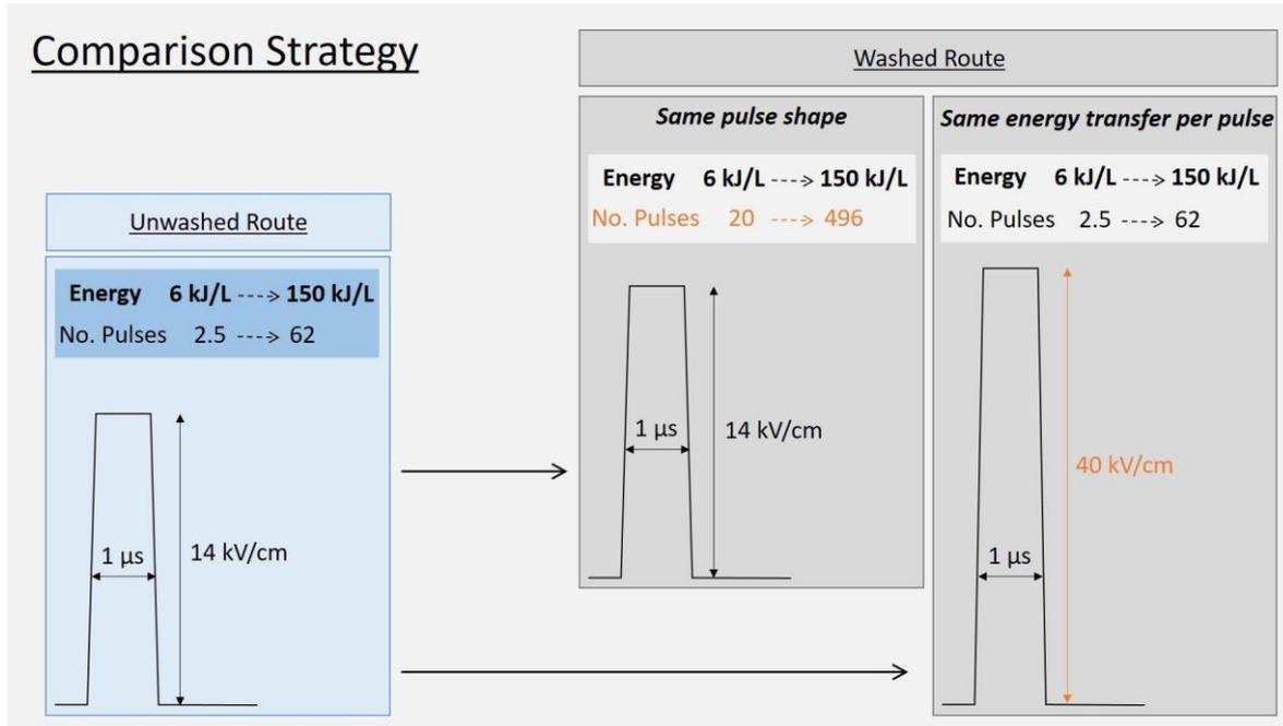
Figure 22: Strategy to compare washed route with the unwashed route. In the washed route the conductivity of the yeast suspension is 8 times lower than in the unwashed route.
