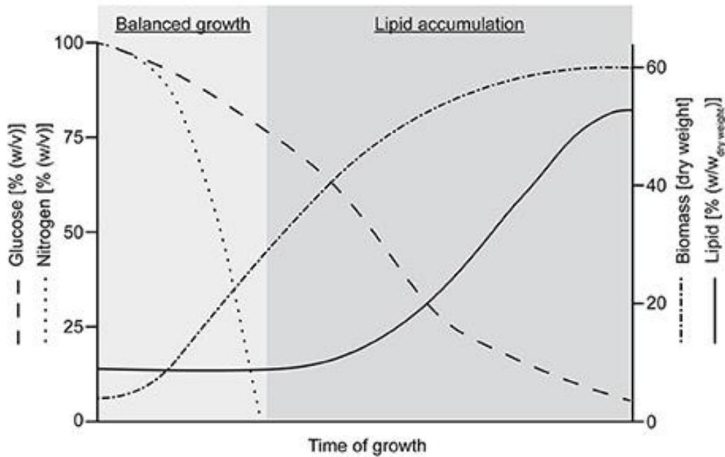
Figure 4: Idealized lipid accumulation profile of a SCO cultivation process with oleaginous yeasts. In the balanced growth phase the medium is initially formulated for optimal biomass formation but in the end of it nitrogen is exhausted and carbon is in excess. In the lipid accumulation phase biomass formation stagnates and the glucose is channelled to storage lipid synthesis. Taken from Ochsenreither et al. (2016).
