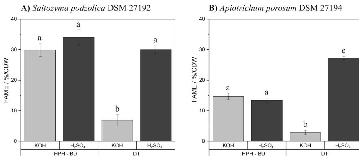
Figure 13: Comparison of KOH and H<sub>2</sub>SO<sub>4</sub> catalysts for FAME production after HPH-BD treatment and direct transesterification (DT) of yeast biomass. % FAME per CDW from *S. podzolica* biomass is demonstrated in (A), while (B) presents the same for *A. porosum*. The standard deviation of three independent experiments are indicated by the error bars. a, b, c illustrate statistical differences ( $p = 0.05$ ).
