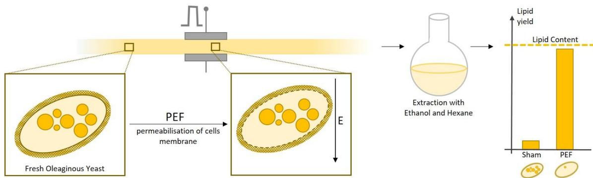
Figure 16: Pulsed electric field treatment performed on fresh yeast biomass induced permeabilisation of cells and greatly improved the yields of subsequent lipid extraction using ethanol and hexane.
