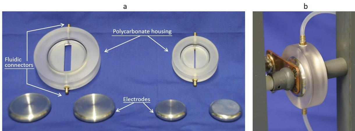
Figure 17: Illustration of the PEF-treatment chambers. (a) Disassembled treatment chambers. The chambers are designed for treating suspensions with conductivities of 1.5 mS/cm (left) and 12 mS/cm (right) with a 50 Ohm transmission-line generator. (b) Illustration of an assembled treatment chamber with the tubes used for the continuous flow of the yeast suspension.
