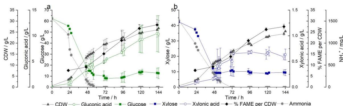
Figure 8: Process plots of established automated continuous feeding with constant sugar excess of about 10 g/L in the fed-batch phase on (a) glucose and (b) xylose. Error bars result from the standard deviation of the experimental set-up in duplicates. CDW, cell dry weight; FAME, fatty acid methyl esters.
