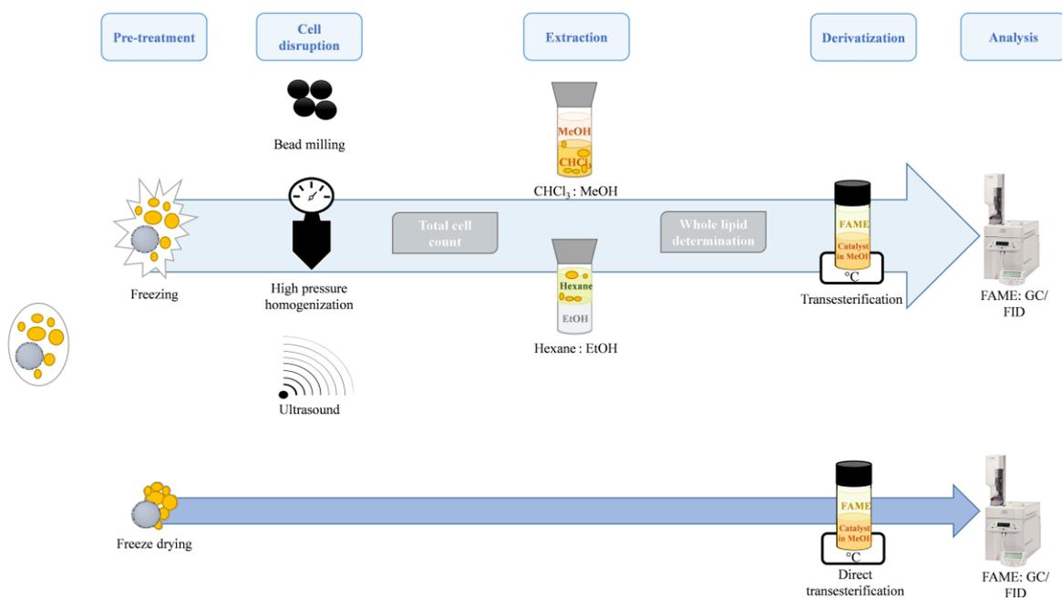
Figure 11: Overview of performed methods for lipid recovery in this paragraph.
