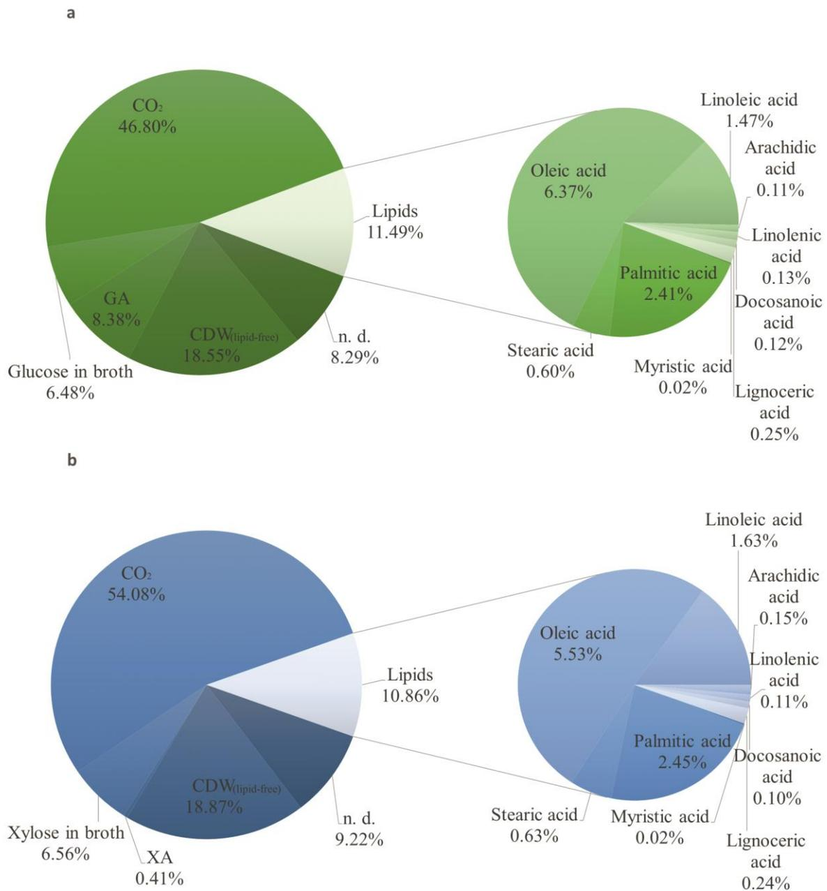
Figure 10: Approximate determination of the overall carbon distribution to process products including by exhaust gas assessed CO<sub>2</sub> emission from automated continuous feed process of *S. podzolica*. a) Approximate percentage distribution of glucose conversion. a) Approximate percentage distribution of xylose conversion. CDW, cell dry weight; n.d., not determined.
