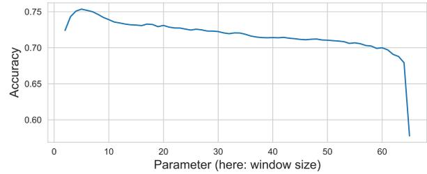
**Figure 10:** Exemplary visualization of the process for obtaining the best parameterization per approach in a brute force manner, here on the example of the proposed feature extraction approach. By testing each plausible parameterization, the best one can be determined, in this case a window size of 5.
