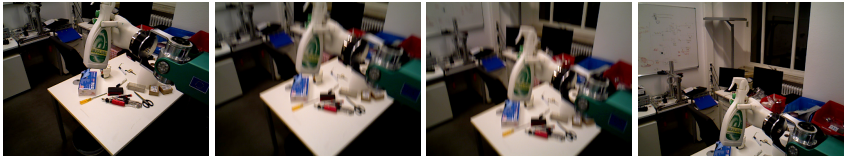
Figure 5.1: Camera images of ARMAR-6's PrimeSense RGB-D sensor while the head is moving at different times. During the gaze shift towards the grasped spray bottle camera images are blurry.
