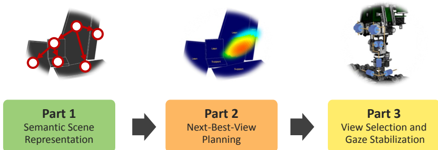
Figure 1.2: The structure of the automatic scene perception approach. The approach starts by describing a semantic scene model built from the current view. The subsequent part determines the NBV to improve the scene model. Finally, a gaze stabilization controller is linked to allow perception during motion. The outline of this thesis follows the structure of the approach.
