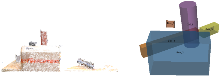
Figure 3.2: An input point cloud and the fitted geometric primitives.
