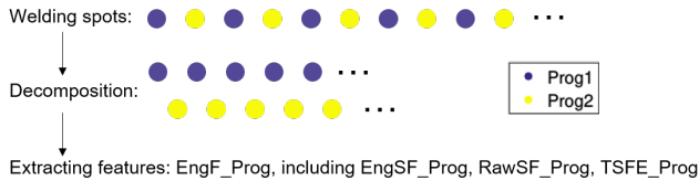
Figure 2.24: Example for generating EngF_Prog with data of Welding Machine 1, modified from [170]. Each dot indicates a welding spot and its data. Purple dots belong to Welding Program 1 and yellow dots belong to Welding Program 2. All single features that form time series on the welding operation level are decomposed into sub-time series, each only belonging to one ProgNo. The Engineered Features considering ProgNo (EngF_Prog) are extracted separately from each sub-time series.
