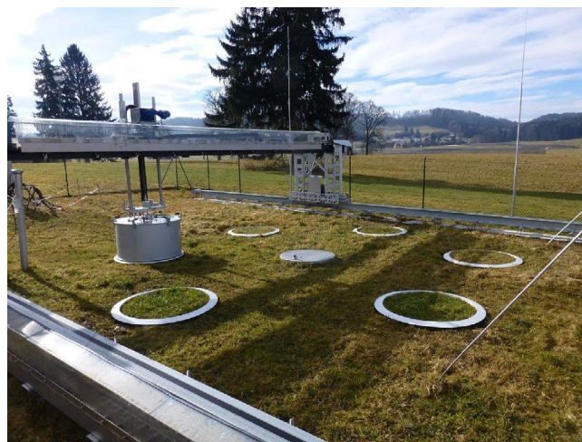
FIGURE 5 The Karlsruhe Institute of Technology Robotic greenhouse has chamber system for mounting on lysimeters at the DE-Fen site within the TERENO (TERrestrial ENvironmental Observatories) network
