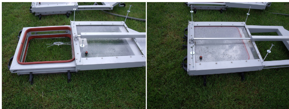
FIGURE 4 Automated greenhouse gas chambers developed by AgResearch (New Zealand). Chamber open (left) and closed (right)
