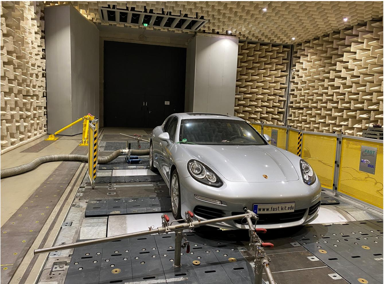
**Figure 2.** VuT mounted on a chassis dynamometer.
