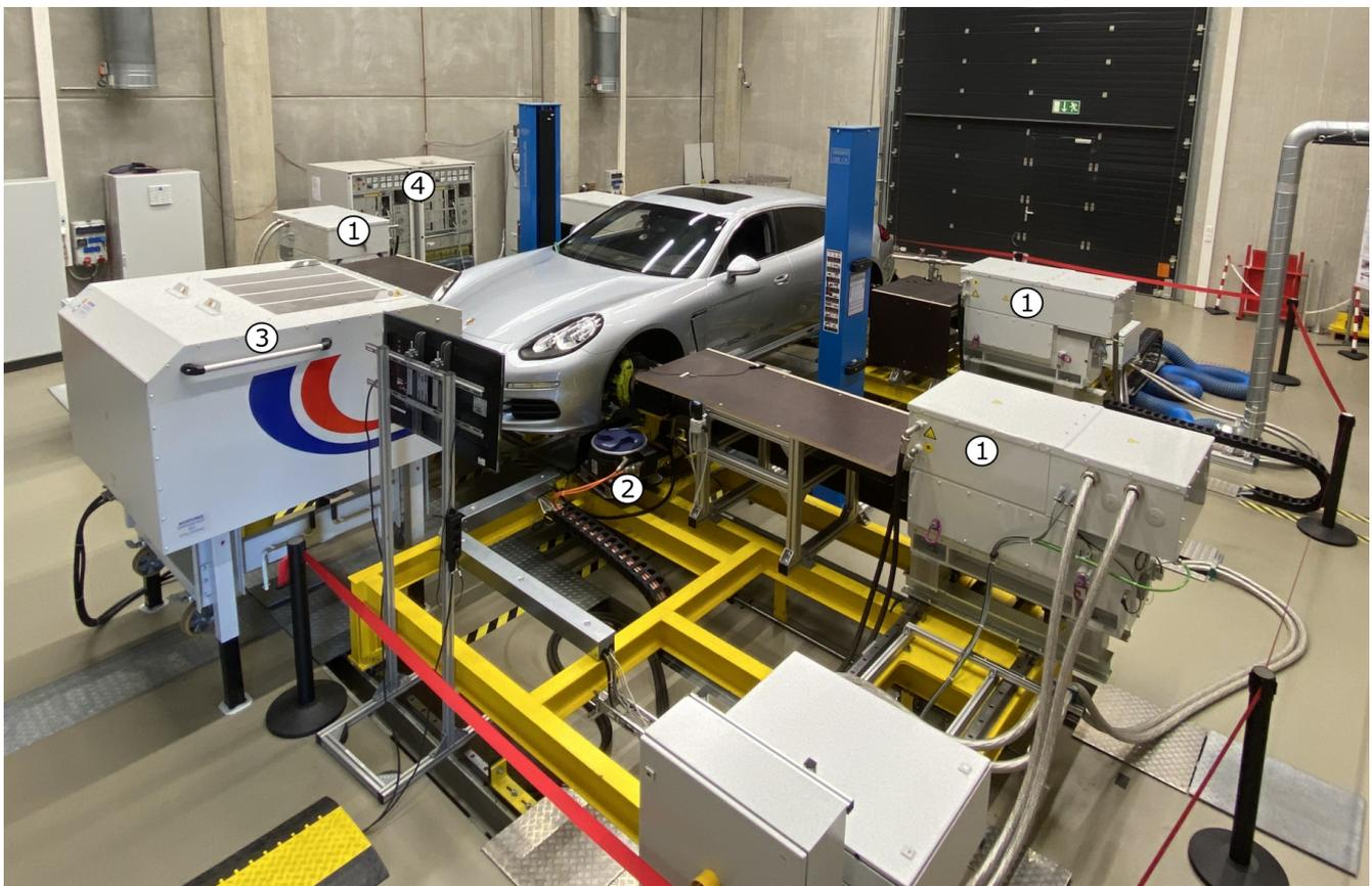
Figure 3. Vehicle-in-the-Loop test bench.
