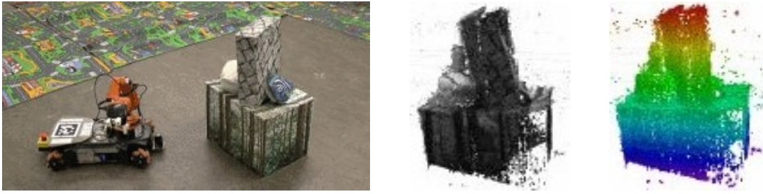
Figure 2.11.: NBV approach for object modeling as presented in Isler et al. (2016) (© 2016 IEEE). Left : Scene of the experiment. Middle : Point clouds of the reconstruction result. Right : Voxelized representation of the object reconstruction result.
