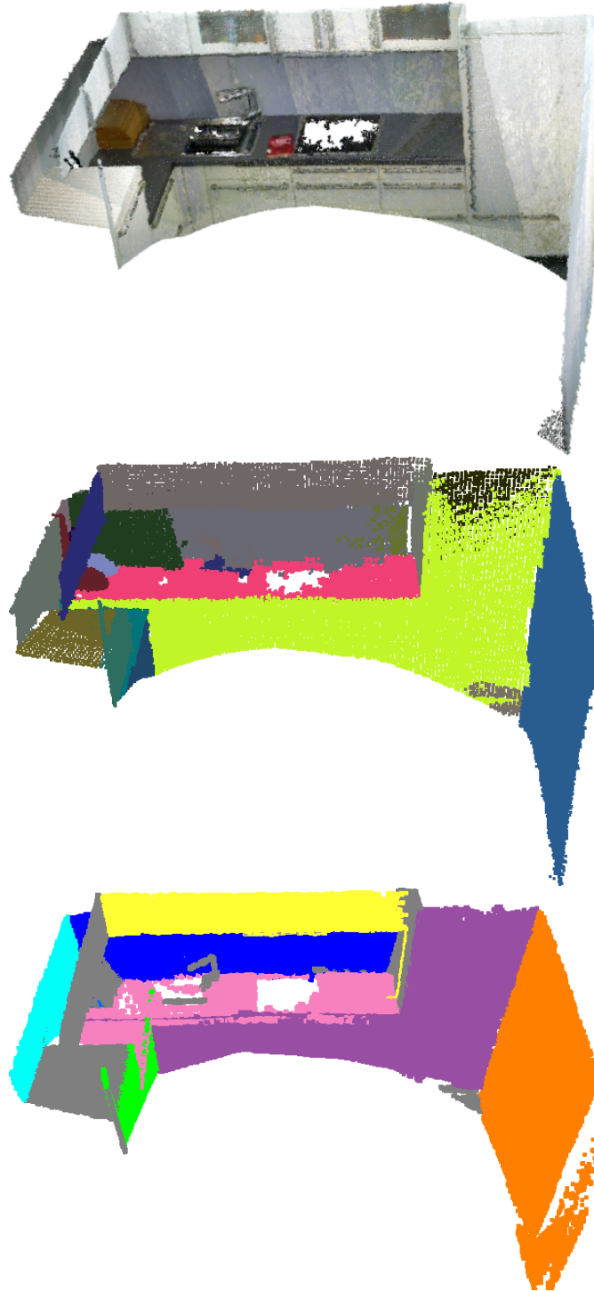
Figure 3.9.: Kitchen scenario as described in Section 3.4.2. Top : The image shows the registered result of the source point cloud. Middle : Multiple views are first registered and then geometric primitives are extracted. Bottom : Primitives are extracted iteratively from consecutive frames. Figures taken from Grotz et al. (2017b) (© 2017b IEEE).
