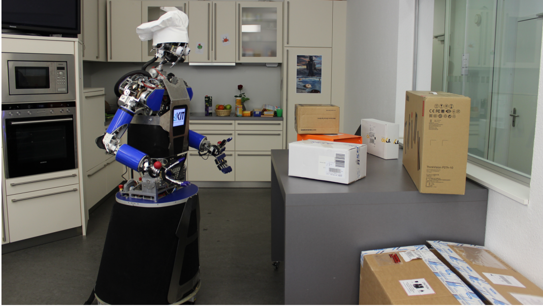
Figure 3.3.: The humanoid robot ARMAR-III in a kitchen environment. The robot does not have any knowledge about the scene. The goal of the experiment is to lift a box from the table. Since both sides of the box are required for executing the manipulation action more than one view is required. Hence, multiple-views are registered with respect to each other and the geometric primitives are fitted.
