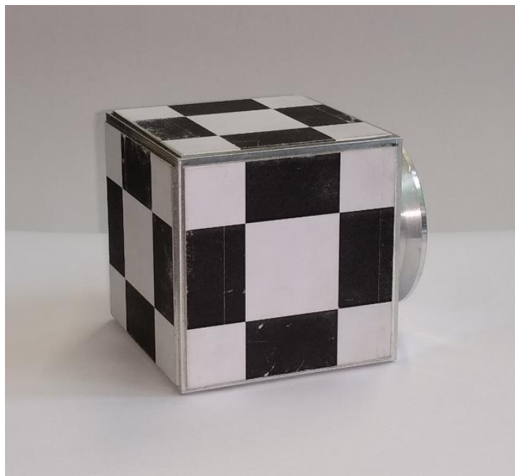
Figure 3: End-effector with chequerboard target
