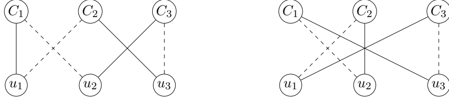
Figure 4.3: Example for two different node-community assignments with existing fixed assignments (dashed) such that there are no two assignments that can be switched to get from one to the other.
