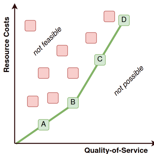
Figure 2.3.: Illustration of a Pareto frontier marked as green line. The green boxes represent allocations which are Pareto efficient. The red boxes represent Pareto inefficient allocations.
