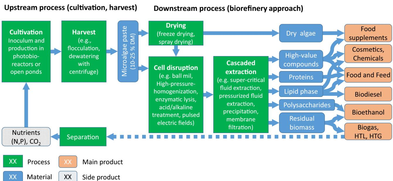
FIGURE 1 Integrated production of fuel and food with microalgae
