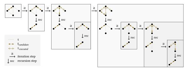
**Figure 7.7.:** Exemplary execution of the provenance algorithm for a change in the topmost model. The transformations present to the current execution of Propagate, as well as the executed and candidate transformations  $\mathfrak{t}_{executed}$  and  $\mathfrak{t}_{candidate}$  are depicted for each iteration (horizontal) and recursion step (vertical). Adapted from [GKB21, Fig. 4].
