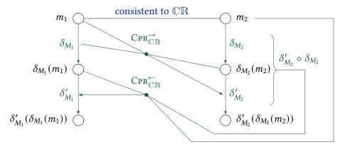
**Figure 6.6.:** Operation of a synchronizing bidirectional transformation execution step. The blue line without arrowheads connects elements that are consistent to  $\mathbb{CR}$ , and green lines with arrowheads indicate changes or consistency preservation execution.
