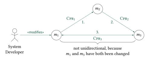
**Figure 4.7.:** Execution of consistency preservation rules of which at least one cannot be unidirectional, because both involved models (circles) have been modified by a user or other consistency preservation rules.
