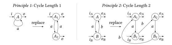
**Figure 7.4.:** Principles to eliminate cycles of length  $\leq 2$  in the transition function of a Turing machine. i and o are placeholders for all incoming and outgoing transitions of a state.
