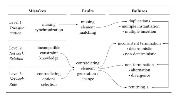
Figure 8.1.: Categorization of mistakes, faults and failures. Adapted from [Kla+19b, Fig. 3].
