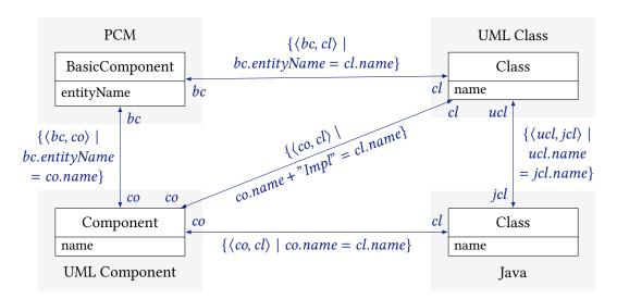
**Figure 9.3.:** Consistency relations between basic components in PCM models, components in UML component models, classes in UML class models and classes in Java models.
