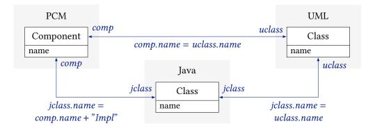
**Figure 1.6.:** Contradicting consistency relations between components in PCM, classes in UML, and classes in Java. The equations are meant to express that for any existing element another element must exist such that the condition is fulfilled.
