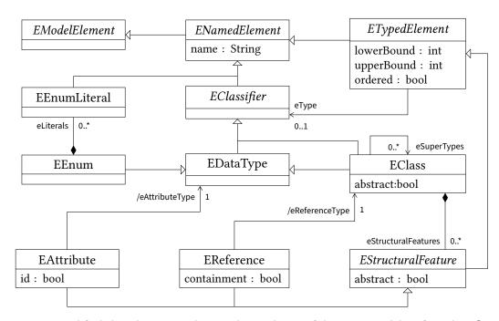
**Figure 2.2.:** Simplified class diagram with central metaclasses of the Ecore modeling formalism [Ste+09, p. 107]. Adapted from [Kra17, Fig. 2.3].
