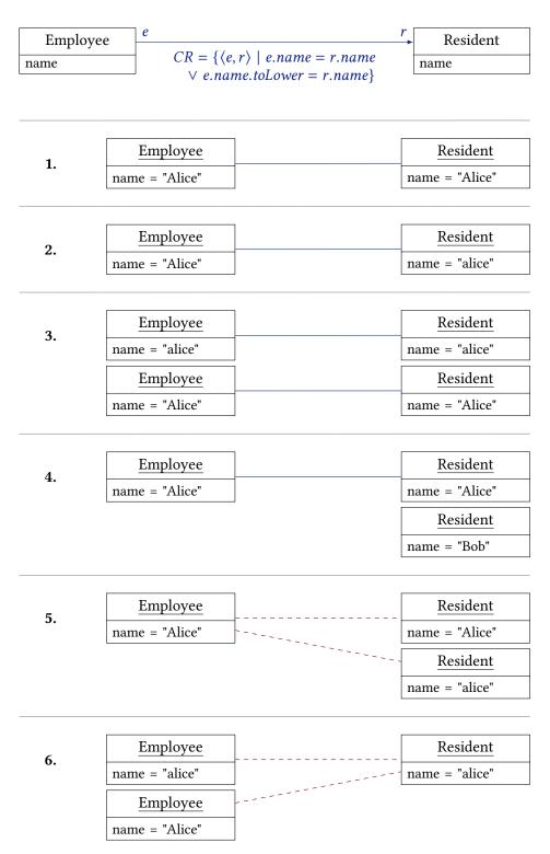
**Figure 4.9.:** A consistency relation between employee and resident and six example model pairs: pairs 1–4 consistent with an appropriate witness structure *W* shown in blue, solid lines, and pairs 5 and 6 inconsistent with an inappropriate mapping structure shown in red, dashed lines. Adapted from [Kla+20, Fig. 2].
