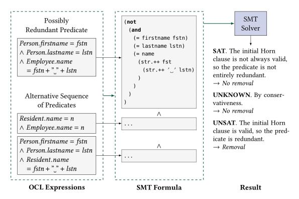
**Figure 5.17.:** Overview of the redundancy test from OCL expressions to the SMT solver results. Adapted from [Kla+20, Fig. 14].
