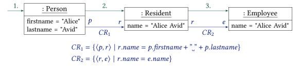
**Figure 5.12.:** Model tuple construction with condition element of  $CR_1$  containing person "Alice Avid" for a consistency relation tree of relations in Figure 5.11. Adapted from [Kla+20, Fig. 7]. Arrows with numbers indicate the order in which elements are created.
