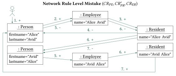
**Figure 8.3.:** Examples for transformation executions based on the consistency relations given in Figure 8.2 with mistakes at each of the three specification levels. Arrows denote user changes and transformation executions with numbers indicating their order and +/- indicating element addition and removal. Adapted from [Kla+19b, Fig. 5].
