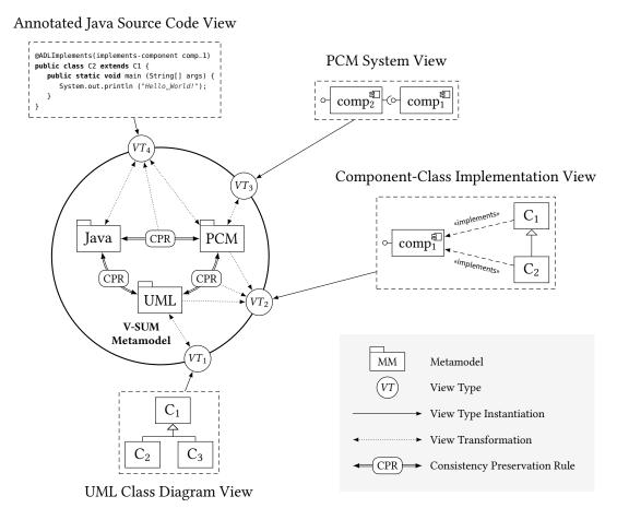
**Figure 2.3.:** Exemplarily V-SUM metamodel consisting of three metamodels for component-based development and exemplarily views derived from them. Adapted from [Lan17, Fig. 4.4].
