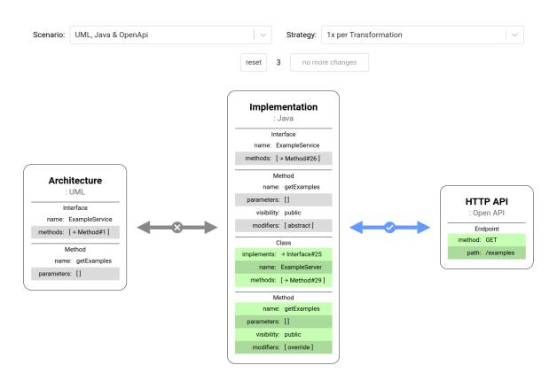
**Figure 7.6.:** Screenshot of a network for an architecture specification, its implementation, and an API specification in OpenAPI [OAPI], which requires multiple execution of the same transformation, developed in the transformation network simulator [GitSim].
