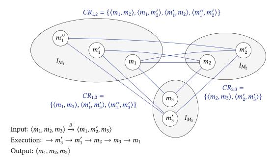
**Figure 5.6.:** Example for rejecting a user change because of consistency relations containing model pairs that are never globally consistent. Small circles denote models, and solid, blue lines relate consistent models.
