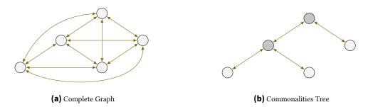
**Figure 11.8.:** Complete graphs as an extreme of transformation network topologies in comparison to the tree topology of a Commonalities specification. Nodes depict metamodels and edges depict transformations. In a Commonalities specification, leaves represent concrete metamodels whereas inner nodes represent concept metamodels. Adapted from [KG19, Fig. 4].
