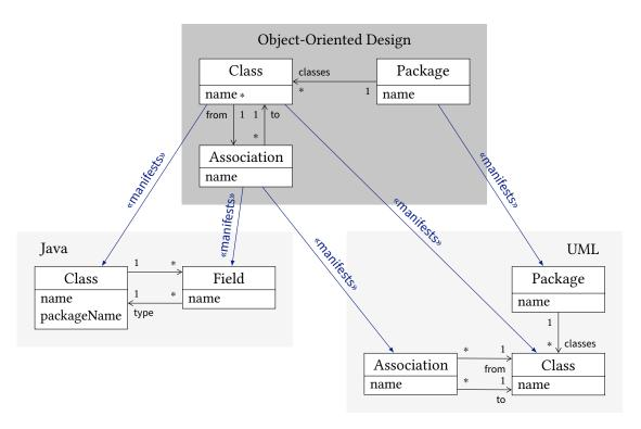
**Figure 11.4.:** Concept metamodel for object-oriented design with a Class, an Association and a Package Commonality and its relations to the concrete metamodels UML and Java with a different representation of associations as fields and packages as attributes of classes in Java.
