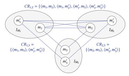
**Figure 5.4.:** Example for obsolete model pairs in consistency relation  $CR_{1,2}$ , which can never occur in a globally consistent model tuple. Small circles denote models, and solid, blue lines relate consistent models.
