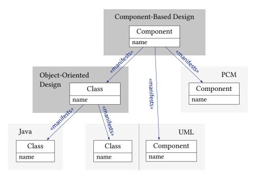
**Figure 11.6.:** Concept metamodels for component-based and object-oriented design and their manifestation relations between each other and to concrete metamodels for the example introduced in Figure 11.1 and extended with components in the UML. Adapted from [KG19, Fig. 3].
