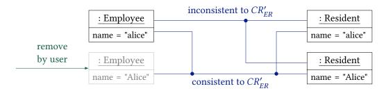
**Figure 6.2.:** Non-alignment of unidirectional relations and preservation rules. Blue lines without arrowheads connect elements that together are consistent or inconsistent to the noted relations. Green lines with arrowheads indicate changes by users or consistency preservation.
