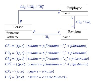
**Figure 5.9.:** Three metamodels with different options for consistency relations. The relation sets  $\{CR_1, CR_1^T, CR_2, CR_2^T, CR_3, CR_3^T\}$  and  $\{CR_1, CR_1^T, CR_2'', CR_2''^T, CR_3, CR_3^T\}$  are compatible, whereas the sets  $\{CR_1, CR_1^T, CR_2', CR_2'^T, CR_3, CR_3^T\}$  and  $\{CR_1, CR_1^T, CR_2, CR_2^T, CR_3, CR_3^T\}$  are not. Taken from [Kla+20, Fig. 4].
