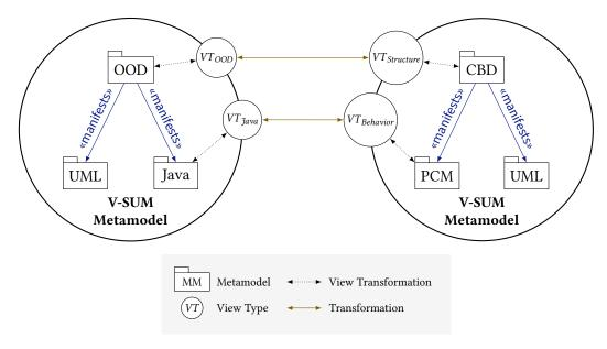
**Figure 11.15.:** Example for the combination of two Commonalities specifications for object-oriented (OOD) and component-based design (CBD) by encapsulation into V-SUM metamodels.
