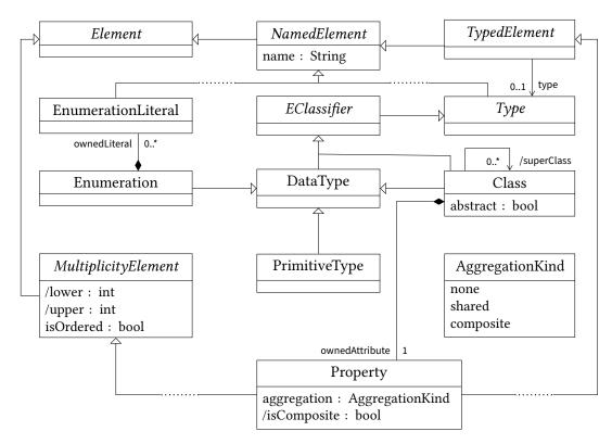
**Figure 2.1.:** Simplified class diagram with central metaclasses of the EMOF modeling formalism [MOF, p. 27]. Dotted lines denote indirect inheritance. Adapted from [Kra17, Fig. 2.2].
