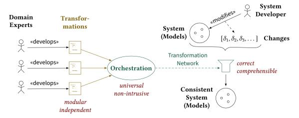
**Figure 1.2.:** The process of specifying and executing a transformation network. Project-specific development artifacts (transformations) are marked orange and the universal application artifacts (orchestration with a resulting transformation network) are marked green. Concrete systems and changes represent runtime artifacts. The assumed and envisioned properties are denoted in red and italics.
