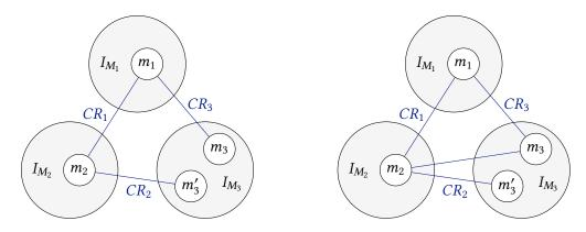
**Figure 4.6.:** Modular consistency relations, which together cannot be fulfilled (left) or which cannot be fulfilled for some of the consistent model pairs (right). Small circles denote models and (blue) lines relate consistent model pairs.
