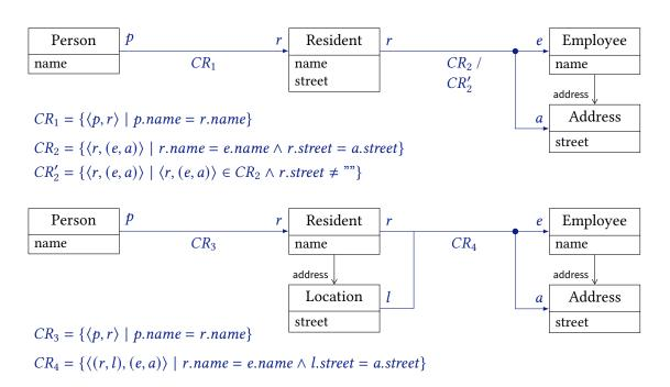
**Figure 5.8.:** Two scenarios, each with two consistency relations: Consistency relations  $CR_1$  and two options  $CR_2$ ,  $CR'_2$  with  $CR_1 \otimes CR_2 \neq \emptyset$  and  $CR_1 \otimes CR'_2 = \emptyset$ , and consistency relations  $CR_3$  and  $CR_4$  with  $CR_3 \otimes CR_4 = \emptyset$  and  $CR_4^T \otimes CR_3^T \neq \emptyset$ . Taken from [Kla+20, Fig. 3].
