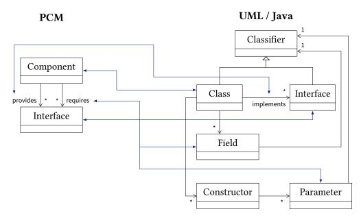
**Figure 1.3.:** Extract of consistency relations between component-based architectures in PCM and object-oriented design in UML/Java according to Langhammer [Lan17]. (Blue) lines with arrowheads indicate that the connected elements share a consistency relation. Properties, such as names, are omitted.
