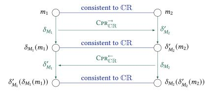
**Figure 6.3.:** Schema for sequencing unidirectional consistency preservation rules after concurrent changes. Circles denote model states, blue lines connect consistent models, and green lines with arrowheads denote the execution of changes or consistency preservation.
