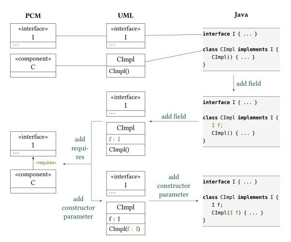
**Figure 7.1.:** Necessity of executing a transformation multiple times. For initially consistent models, the Java code is changed, requiring the UML and PCM models to be updated accordingly. Blue lines without arrowheads connect initially corresponding elements, and green lines with arrowheads indicate changes performed by a user or consistency preservation.
