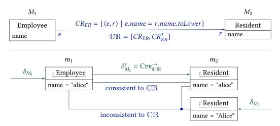
**Figure 6.4.:** Example for non-transformability when sequencing the application of unidirectional consistency preservation rules and concurrent changes. Blue lines without arrowheads connect elements that are (in-)consistent to  $\mathbb{CR}$ , and green lines with arrowheads indicate changes.
