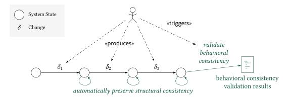
**Figure 3.1.:** Proposed process for continuously and automatically preserving structural and explicitly checking behavioral consistency.
