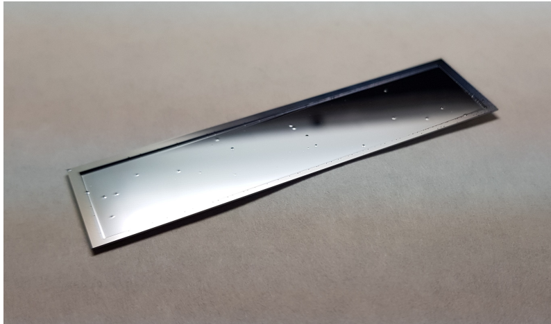
Figure 9.1: Backside of a 7.5 cm long, selectively thinned H35Demo module.
