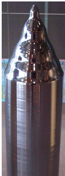
Figure 2.3: Mono-crystalline silicon is produced as cylinders, so-called boules, which can be cut into wafers. (From [12])
