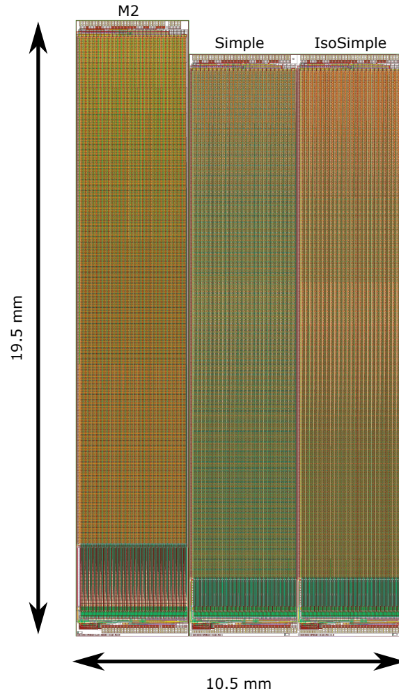
Figure 11.1: The layout of ATLASpix1. All three matrices have bond pads on the top and bottom edge. Simple and IsoSimple share most characteristics, M2 differs from them considerably.
