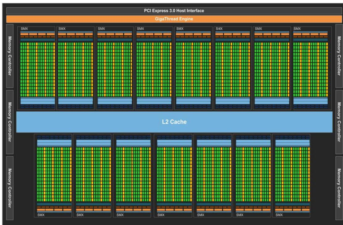
Figure 4.7: NVIDIA K40c GPU GK110 Architecture
