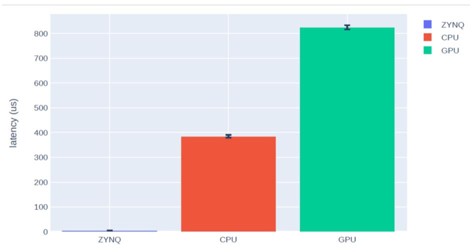
Figure 7.19: one-step episode error bar compared with ARM, CPU and GPU
