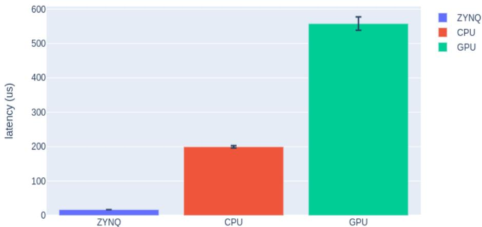
Figure 9.20: The comparison between CPU GPU and Zynq.
