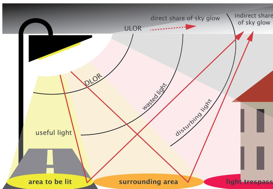
DLOR (downward light output ratio) = proportion of light emitted into the lower half space
