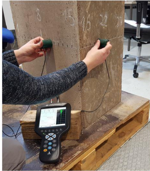
Figure 3.6: Acquisition process on the concrete block. The source and the receiver are positioned on the spotted points and the signal recorded viewed on the handle unit Müller (2020).
