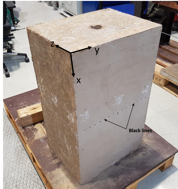
Figure 3.1: Concrete block with a pipe of 5 cm in the middle. Different measurement points are spotted as small black lines. They are equally spaced.
