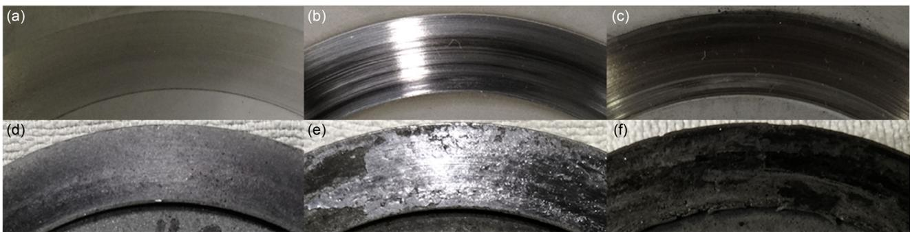
**Fig. 11** Steel disk (top) and friction lining (bottom); after running-in (a, d); after fade (b, e); and after recovery (c, f).
