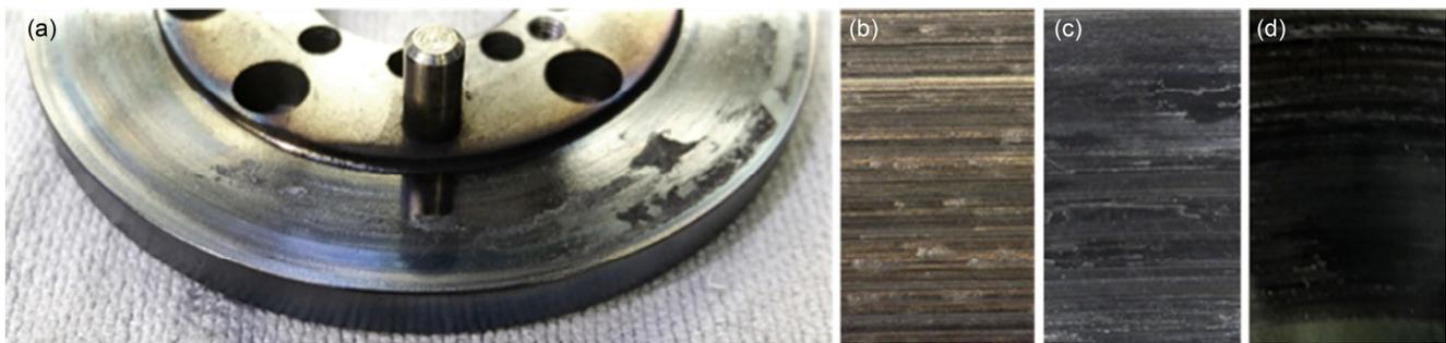
**Fig. 17** More examples of material transfer. Pictures of (a, b) steel disks of mass pressed; (c) wound; and (d) sintered metal friction linings.
