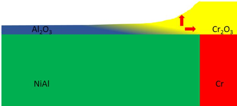
Figure 8.18: Schematic view of NiAl-Cr with oxide scales. Arrows show direction of increasing Cr concentration.
