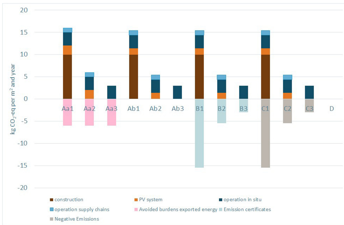
Figure 3: Greenhouse gas (GHG) emissions and GHG emission reductions of the fictive building according to the four approaches and three variations.
