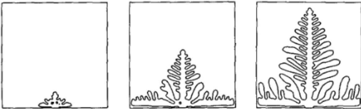
*Figure 3.2: Realistic needle-like dendritic morphology simulated via phase-field method. Reprinted from Kobayashi et al. [91] with permission.*
