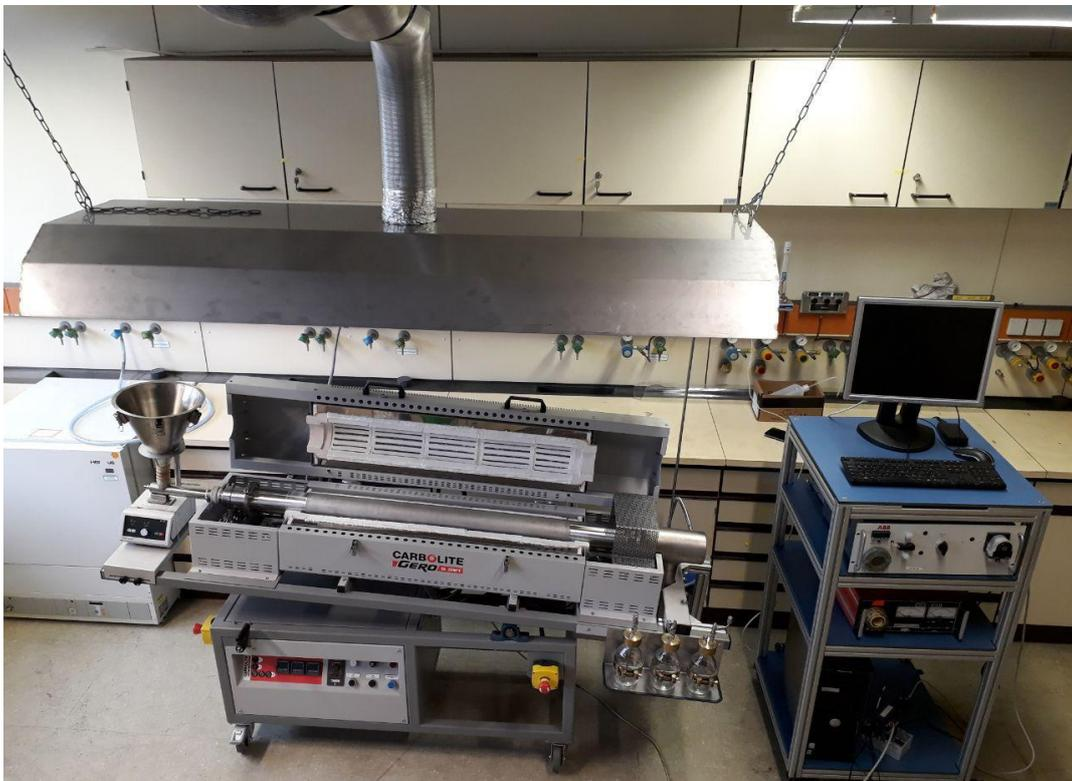
Figure 4.1 Rotary-drum reactor used in the experimental procedure
