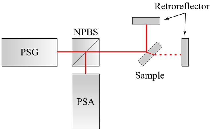
**Figure 1.1:** Schematic of the retroreflex ellipsometer in the reflection and transmission configurations, showing the polarization state analyzer (PSA), polarization state generator (PSG) and non-polarizing beam-splitter (NPBS).
