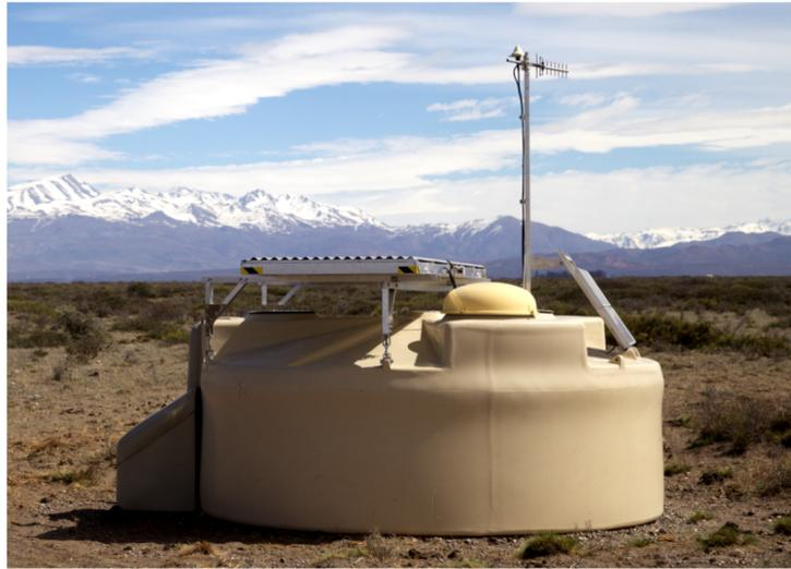
Figure 3.6.: Photography of an SSD on top of the WCD. Image taken from [31].
