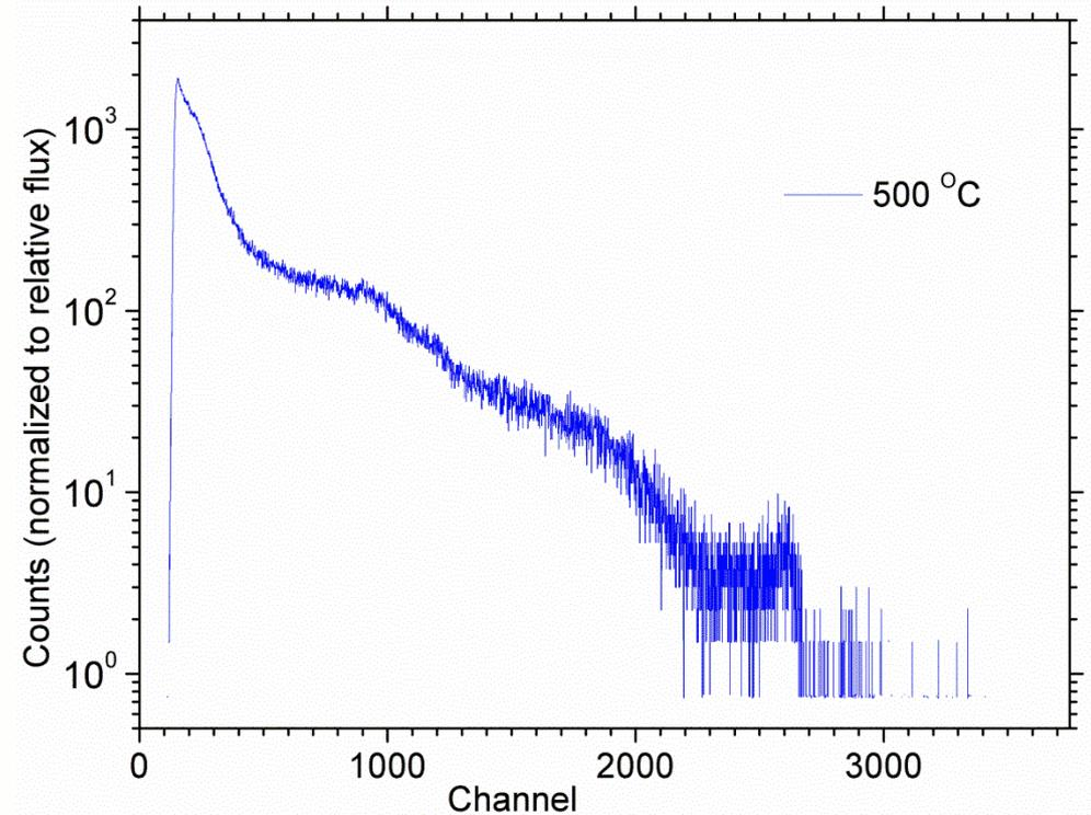
**Even at 500 °C spectroscopic behaviour is retained to some extend.**
