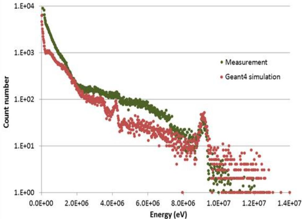
Measured and modeled (GEANT-4) pulse height spectrum under irradiation with 14 MeV neutrons
