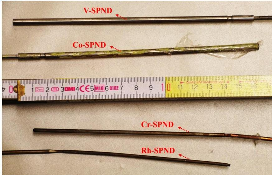
Typical examples of commercially available SPND for fission reactors
