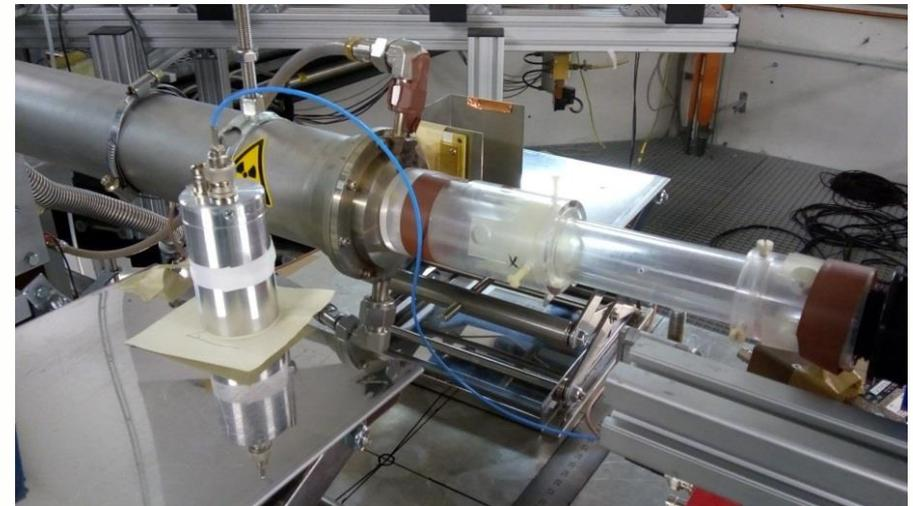
Test rabbit: Nb cylinder closed with Al plugs, Au/Cr/CeO<sub>2</sub> powder filling, PE carrier
