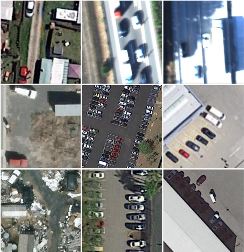
**Figure 1.2:** Illustration of typical challenges occurring in aerial imagery. First row: image noise<sup>1</sup>, motion blur<sup>2</sup> and illumination<sup>2</sup>. Second row: low resolution<sup>3</sup>, high intra-class variance<sup>1</sup> and low inter-class variance<sup>1</sup>. Third row: intricate background<sup>3</sup>, partial occlusion<sup>1</sup> and shadow<sup>1</sup>.
