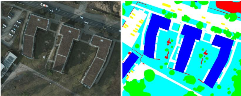
**Figure 4.6:** Example patch of the Potsdam dataset (left) and the corresponding semantic labeling mask (right) with pixel-wise semantic annotations of six categories: *impervious surface* (white), *building* (blue), *low vegetation* (cyan), *tree* (green), *car* (yellow), and *clutter* (red).
