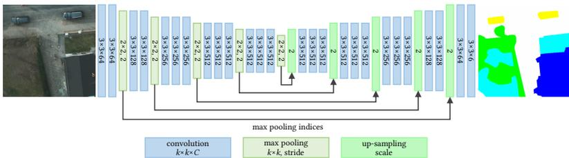
**Figure 6.7:** Schematic structure of SegNet, which is comprised of an encoder and decoder network. The topology of the encoder is identical to the convolutional part of VGG16, while the topology of the decoder is in essence the mirrored encoder. Non-linear up-sampling is performed by using max pooling indices that encode the positions where to map the values of the preceding feature map as shown in Figure 6.8.
