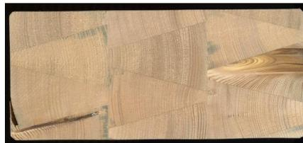
*Figure 2 Layered LST cross-section (120 x 270 mm, illustration turned by 90°) with 3 LST layers*
