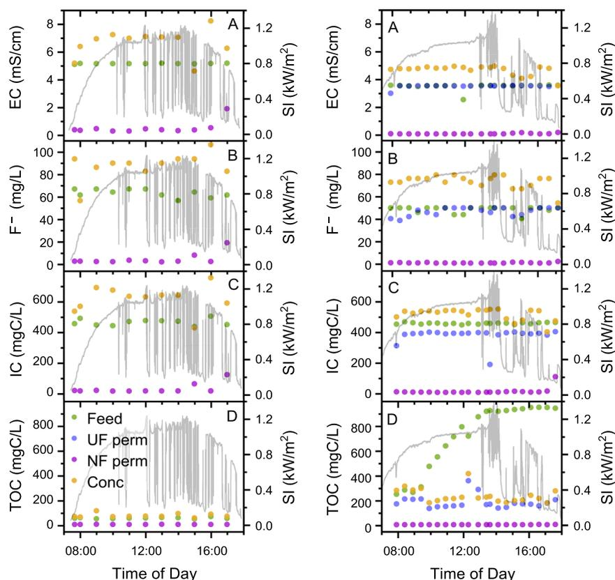
**Fig. 4** Water quality as a concentration of fluoride, electrical conductivity, inorganic carbon and total organic carbon obtained with NF90 in Mdori (left, **a–d**) and Ngare Nanyuki (right, **a–d**) waters
