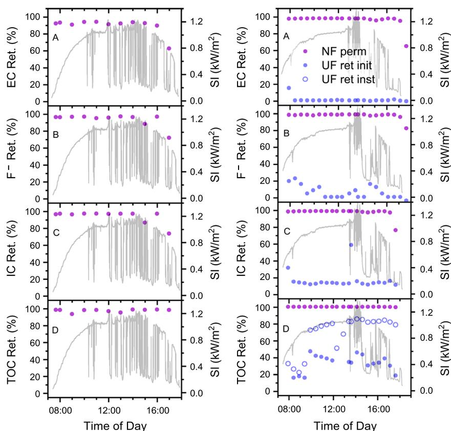
**Fig. 5** Solute retention by UF and NF (NF90) for Mdori (left, **a–d**) and Ngare Nanyuki (right, **a–d**) waters
