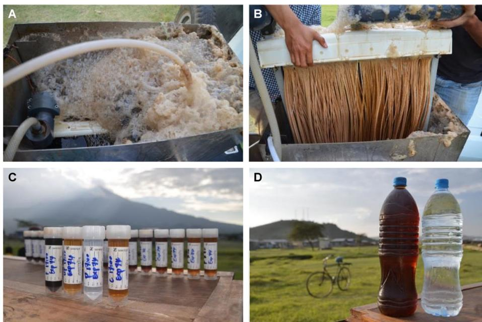
**Fig. 7** Organic matter removal in Ngare Nanyuki: **a** foam development in feed tank, **b** organic matter deposition on UF hollow fibre membranes, **c** samples at the end of the day: feed tank, UF permeate, NF permeate and concentrate and **d** feed and product water (© Schäfer)
