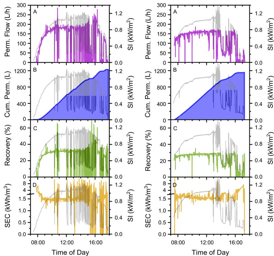
**Fig. 3** System performance results for the NF90 membrane in Mdori (left, **a–d**) and Ngare Nanyuki (right, **a–d**) waters
