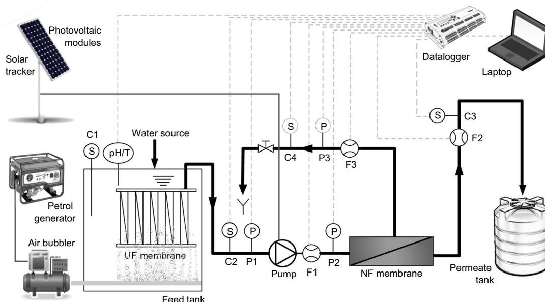
**Fig. 9** Schematic of the renewable energy-powered membrane system (C1 feed sample, C2 UF permeate sample and sensor, C3 NF permeate sample and sensor, C4 concentrate sample and sensor, Fi flow metres, Pi pressure sensors)
