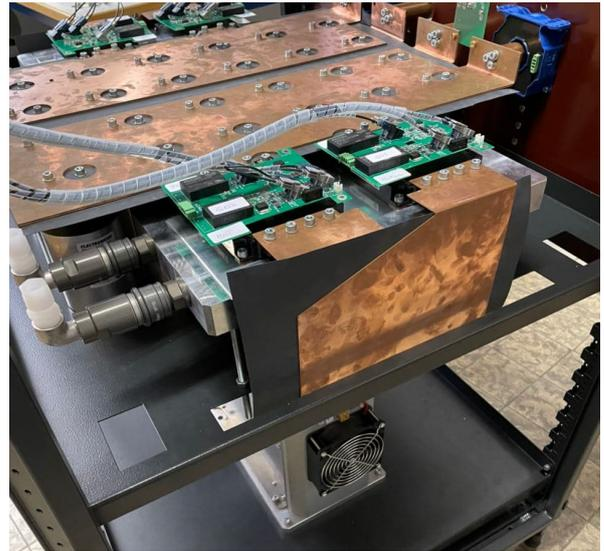
Fig. 7: Setup of the 500 kW DAB
