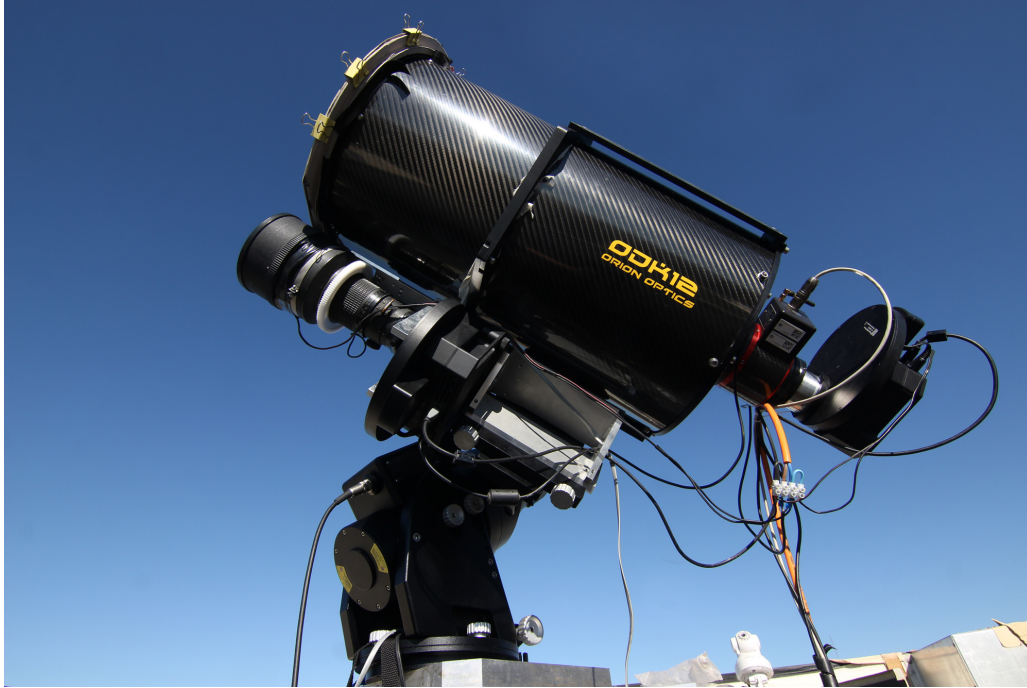
Figure 7. The current FRAM setup with the narrow-field system on the top and the wide-field system on the bottom.
