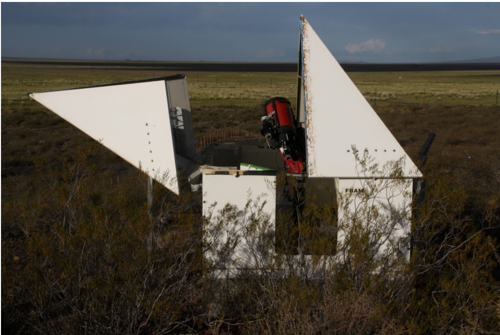
Figure 6. The FRAM enclosure with one half open and one closed. Inside is an older version of the FRAM setup with the Meade SCT and Paramount ME mount.
