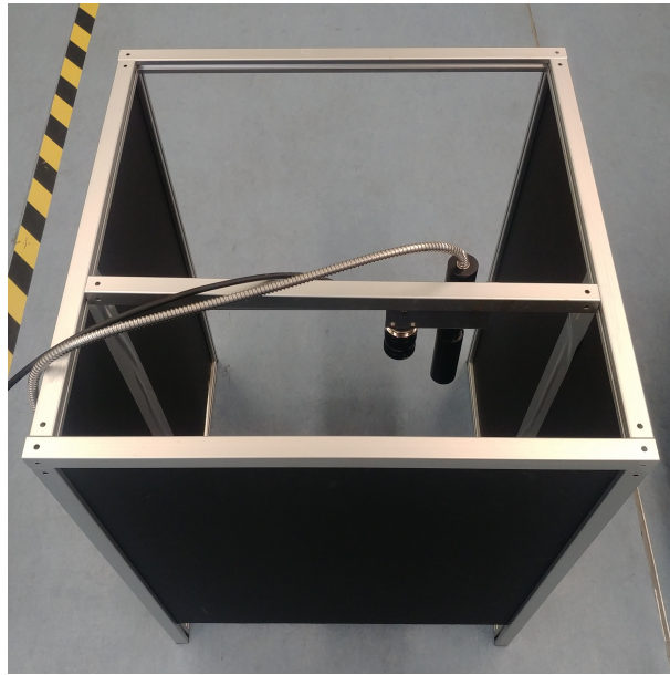
Figure 10.7: The camera and collimator for the illumination were attached to a frame. The camera was connected to a computer via a USB 3.0 cable. The collimator was connected to the xenon light source via an optic fiber. Black plastic panels were included into the frame to minimize the influence of stray light on the experiments. The panels also prevented blood from spattering across the lab in case of a malfunction of a connector.
