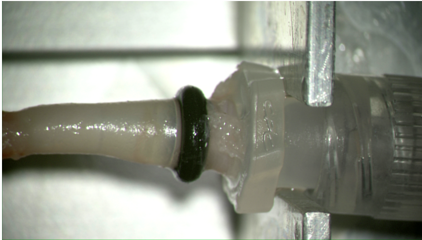
Figure 10.5: The aorta was attached to a barbed nozzle. It was pulled on it and then an o-ring was put over it to firmly press on it. A small amount of glue was dispensed on the aorta behind the o-ring to glue it to the connector. Both steps (o-ring and glue) prevented leakage and provided mechanical stability so the aorta cannot detach from the connector.
