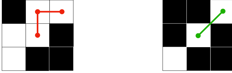
Figure 8.3: To the left a stairway like connection and to the right its correction is visualized. The left figure is used as template to detect stairway like connection in the raw centerline. To the left an incorrect measurement due to a step-like connection with a distance of 2, to the right the corrected centerline with a measured distance of \sqrt{2} . Both images are adapted from [172] published under the Creative Commons Attribution 4.0 License.
