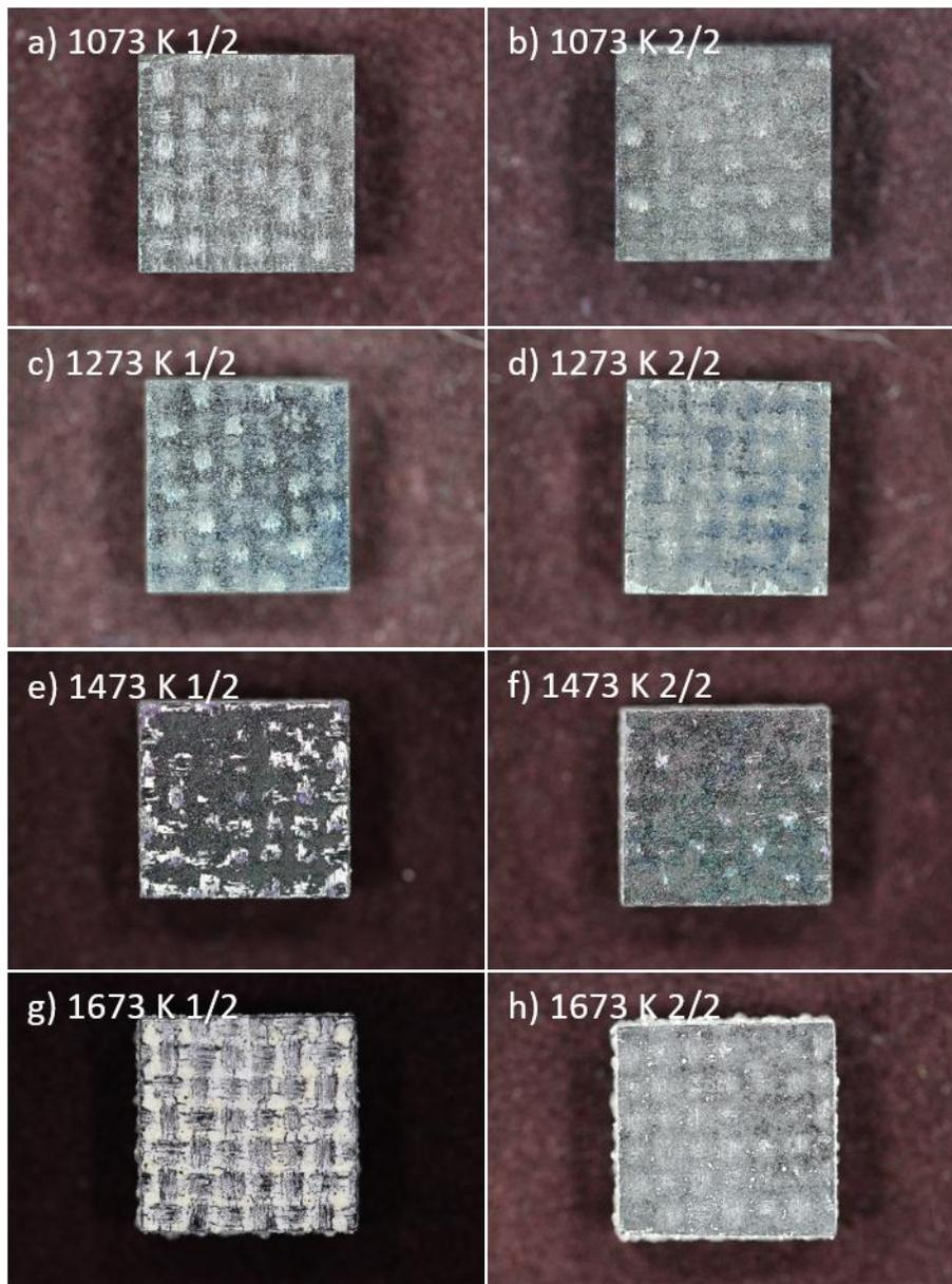
**Figure 8.26:** ZrB<sub>2</sub>-SiC/Si-C-N composites after isothermal oxidation at a), b) 1073 K, c), d) 1273 K, e), f) 1473 K and g), h) 1673 K in O<sub>2</sub>/Ar-atmosphere (p<sub>O<sub>2</sub></sub> = 0.2 bar) for 100 h. Both sample sides are shown. The edge length of the samples corresponds to 10 mm.
