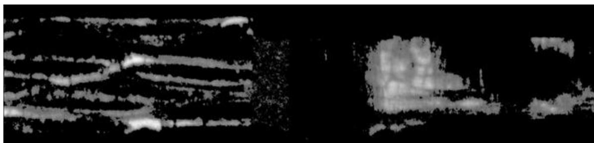
**Figure 8.1:** Neutron tomography image of a ZrB<sub>2</sub>-SiC/Si-C-N composite. The sample was prepared with an orientation of the SiC-fiber preform perpendicular (left) and parallel (right) to the image plane. The shorter dimension corresponds to an edge length of 1 mm. ZrB<sub>2</sub>-rich Si-C-N matrix appears bright.
