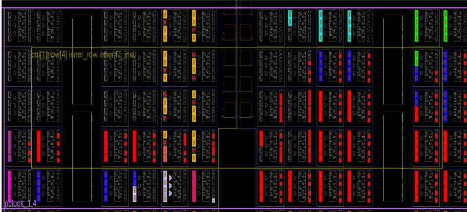
Fig. 4: V-FPGA tile (type 9) placed using the manual placement strategy. Multiplexers of the PSM’s top, right, bottom and left side are marked sky blue, green, dark blue and yellow. The CLB is located at the bottom with the LUT, two internal multiplexers and D-flipflop colored in white. Red color represents the configuration units of the tile. Blue blocks at the bottom depict write connection boxes, whereas read connection boxes make up remaining logic around the LUT.
